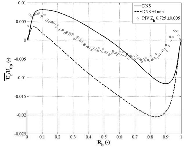
Figure 2: Comparison of the DNS model with the PIV results for the radial velocity component.
