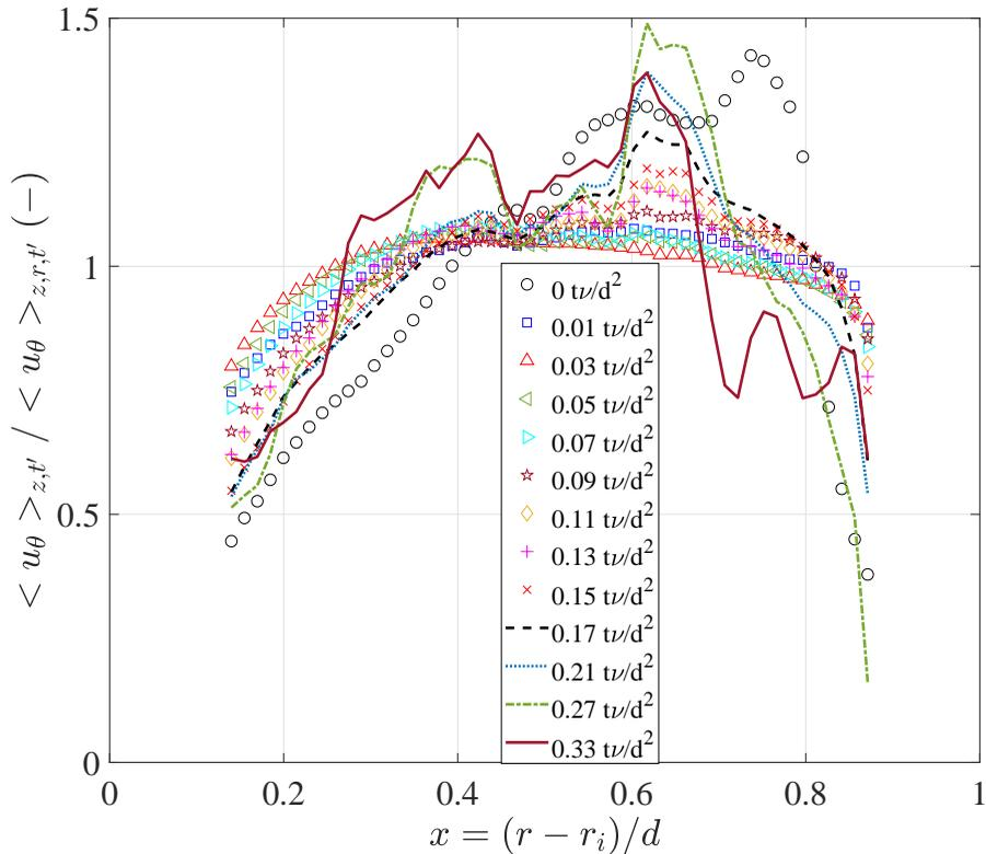
Figure 10: Radial profile of azimuthal velocity averaged axially and over time, for  $t' = (i - 5fd/u_\theta) : (i + 5fd/u_\theta)$ , and normalised with its spatial mean value at  $Re_o = 17300$ . The time represents the instant at which the profile was extracted from the moment decay started.
