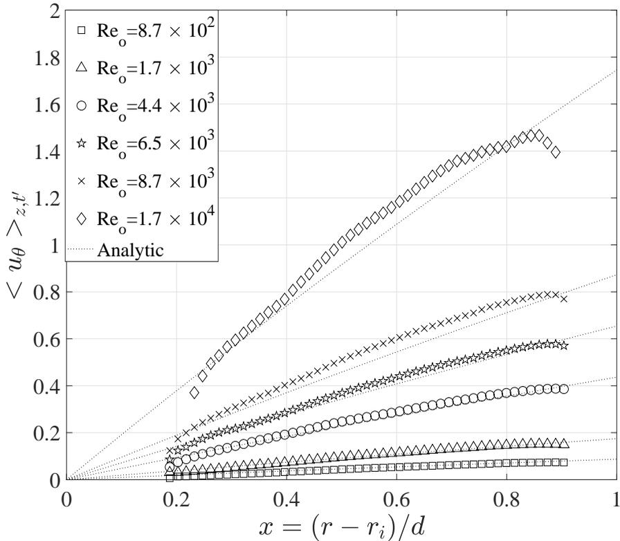
Figure 6: Azimuthal velocity at the instance at which decay starts for different  $Re_o$ . It is averaged axially and at each instant of time with  $t' = (i - 5fd/u_\theta) : (i + 5fd/u_\theta)$ . The vertical red line points towards the inflection point observable at the presented Reynolds number.
