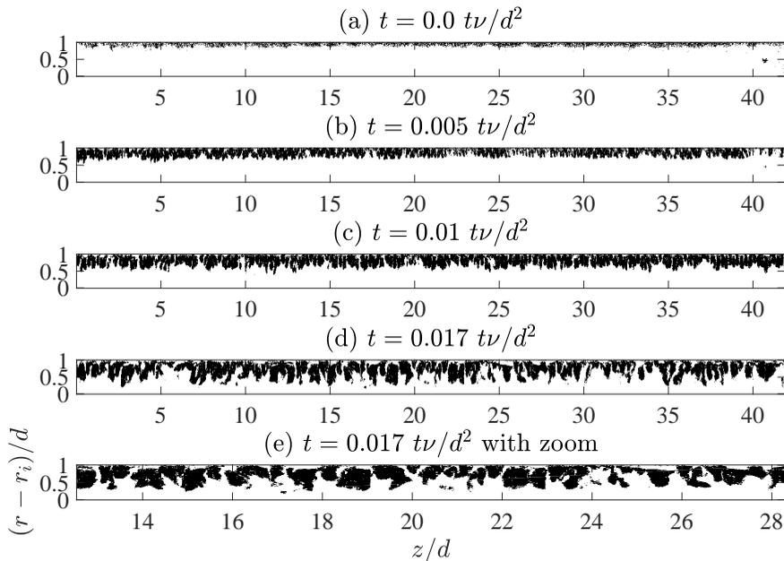
Figure 1: Binarized instantaneous images presenting growth of vortical structures at different times-steps for the  $Re_o = 1700$  over the whole axial height ( $z$ ) of the TC system. The x and y labels are the same for all sub-figures, as in (e).
