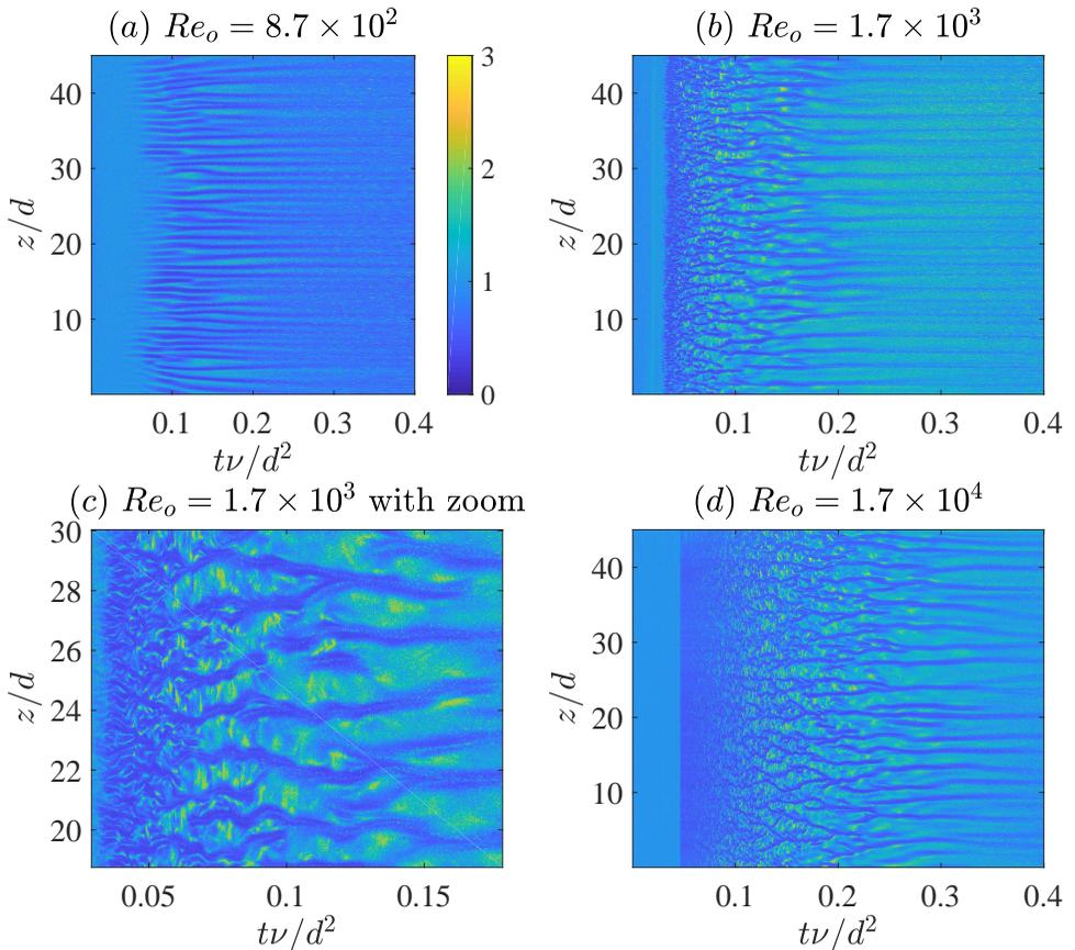
Figure 2: Space-time diagram of the light intensity taken along  $z$  near the outer-cylinder for increasing outer Reynolds number with a stationary inner cylinder.
