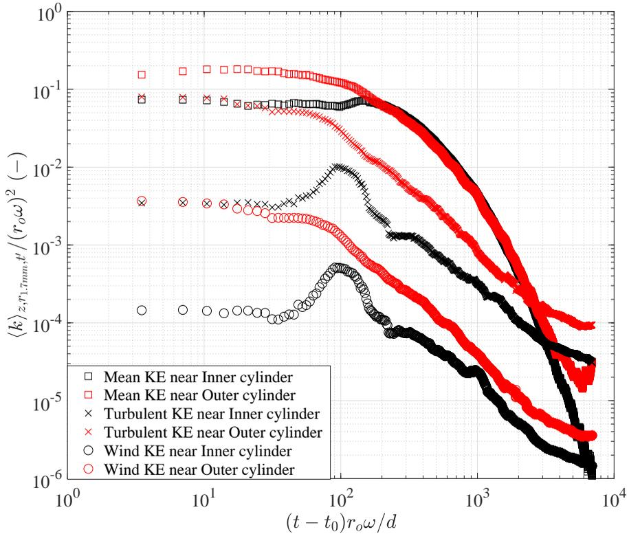
Figure 8: Temporal evolution of the dimensionless mean, turbulent and wind KE at  $Re_o = 17300$  when radially averaged near inner (black markers) and outer (red markers) cylinder. These are averaged axially, radially around the inner cylinder (black markers) and outer cylinder (red markers) over 1.7 mm and at each instant of time with  $t' = (i - 5fd/u_\theta) : (i + 5fd/u_\theta)$ . The  $t_0$  represents the time at which the stop occurs.
