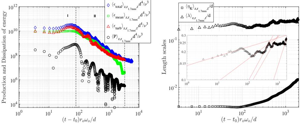
Figure 9: Temporal evolution of the production and dissipation of energy and two length scales at  $Re_o = 17300$ . The insert in b presents the multiple power laws observed in the Taylor microscale. These are averaged axially, radially around the center of gap-width over 1.7 mm and and at each instant of time with  $t' = (i - 5fd/u_\theta) : (i + 5fd/u_\theta)$ . The  $t_0$  represents the time at which the stop occurs.
