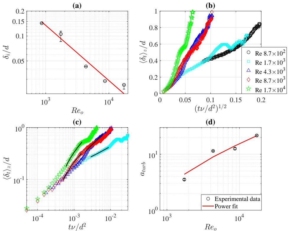
Figure 3: Initial size of the vortex (a), their growth in plot (b) and logarithmic scale (c), and proportionality constant as a function of  $Re_o$  (d). The legend in part (a) is similar to that in (d), and the one in (b) represents (c) as well. In sub-figure (c) symbol represents experimental data and line of the black colour represent fitted curve for the respective  $Re_o$ .
