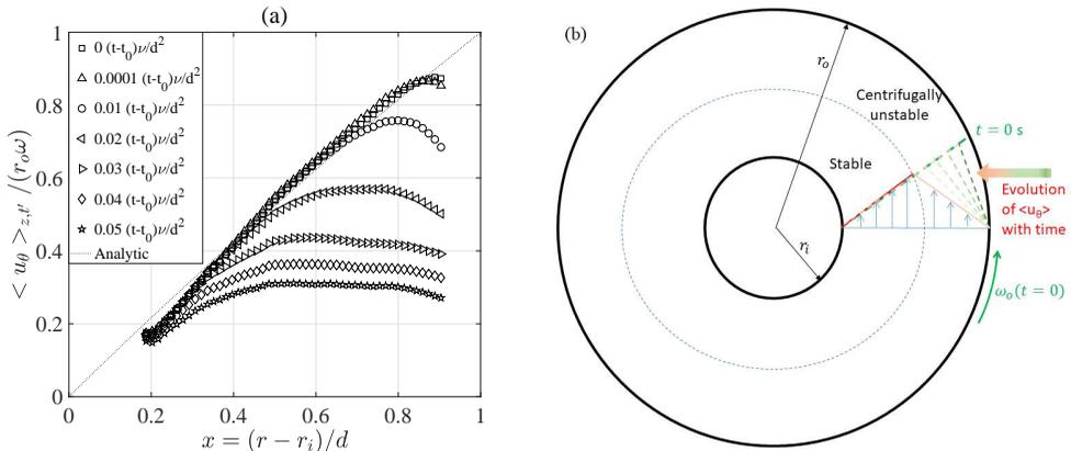
Figure 5: Radial decay process observed experimentally at  $Re_o = 1700$  (a) and its theoretical explanation (b). In (a) mean azimuthal velocity is averaged axially and at each instant of time with  $t' = (i - 5fd/u_{\theta}) : (i + 5fd/u_{\theta})$ . The dotted line represents the analytic laminar profile. The  $t_0$  represents the time at which the stop occurs.
