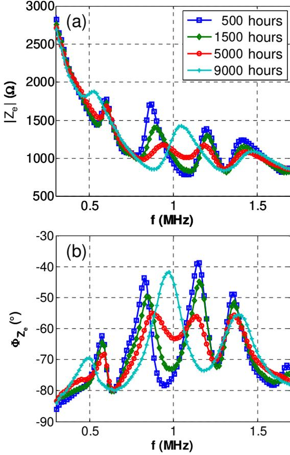
Figure 3: EMI measurements versus the frequency, in the bandwidth of the transducer, centered at  $f_0 = 1$  MHz:
