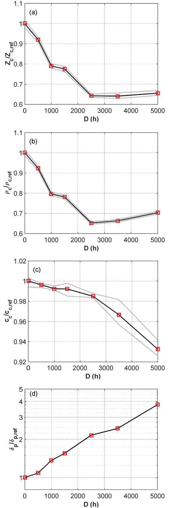
Figure 4: Normalized acoustical parameters versus the ageing duration, from 500 to 5000 h: (a) Acoustical impedance  $Z_c/Z_{c,ref}$ , (b) Density  $\rho_c/\rho_{c,ref}$ , (c) Wave velocity  $c/c_{c,ref}$ , (d) Loss parameter  $\delta_c/\delta_{c,ref}$ .
