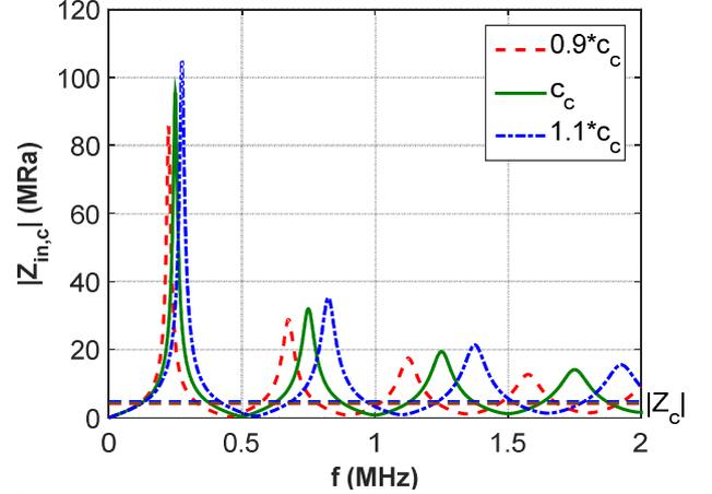
Figure 2: Sensitivity of the wave velocity  $c_c$  on the input impedance of a composite plate  $|Z_{in,c}|$  (eq. (6)), with a wave velocity  $c_c = 3000$  m/s, a density  $\rho_c = 1500$  kg/m<sup>3</sup>, a loss parameter  $\delta_c = 3\%$  and a thickness  $t_c = 3$  mm.
