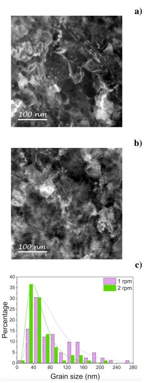
Figure 8: Dark field TEM micrographs of UFG CuSn8 processed by HPT ( $\gamma = 380$ ) at 1 rpm (a) and 2 rpm (b), and corresponding grain size distributions (c), 2mm samples.
