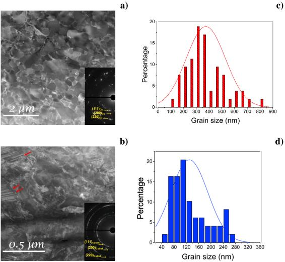
Figure 2: Dark field STEM images of Cu (a) and CuSn8 (b) processed by HPT (800 $<\gamma<$ 1200, 1mm samples, 1 rpm) with corresponding SAED patterns (insets) Arrows in b) point twins resulting from SPD. Corresponding grain size distributions (c) and (d) were estimated from these images.
