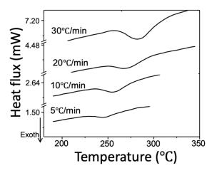
Figure 3: DSC thermograms at different heating rates of Cu processed by HPT (1mm samples, 1 rpm).
