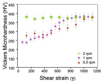
Figure 5: Micro-hardness as a function of the shear strain for CuSn8 processed by HPT at various rotation speeds (2mm samples).
