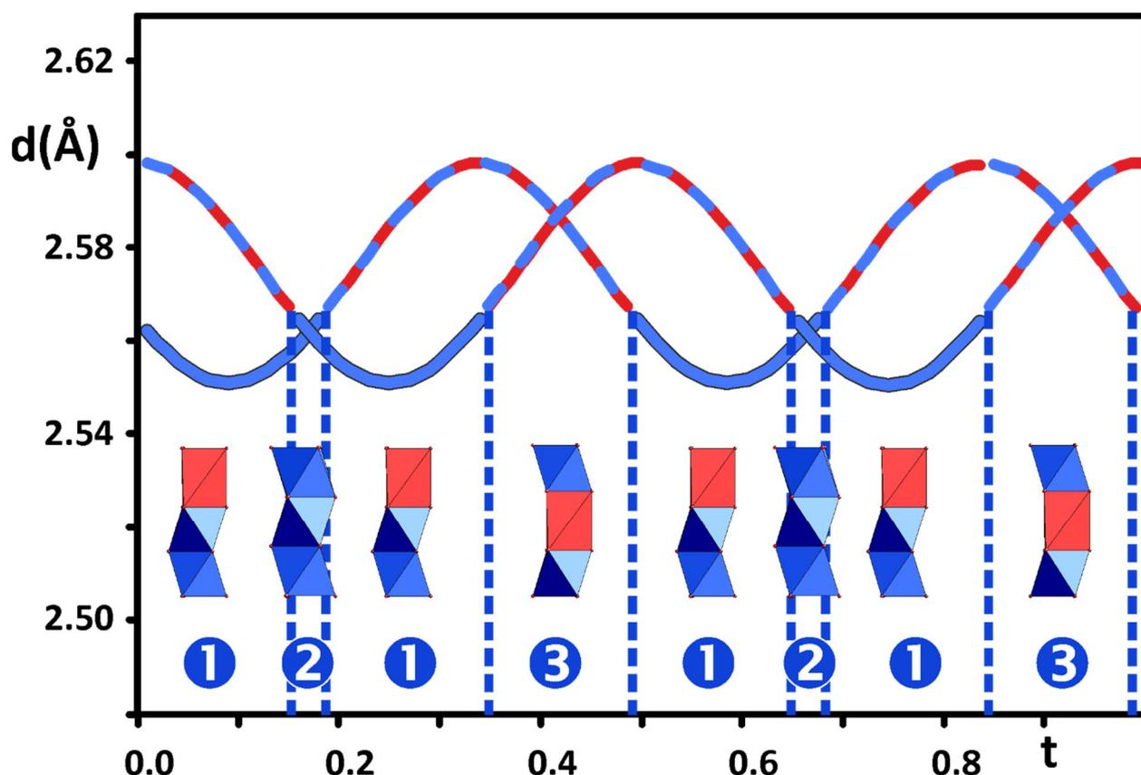
**Fig. 10:** Distances between M and M' sites along  $c$  for the incommensurate crystal of sample Crystal II : Evolution versus the internal  $t$  parameter of the M-M (blue curves) and M-M' (dashed red – blue curves) distances for three metallic first neighbors within A or B chains. Three different
