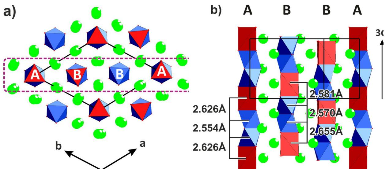
**Fig.6** Structure of the commensurate oxide  $\text{Sr}_{4/3}(\text{Mn}_{0.606}\text{Co}_{0.364}\square_{0.03})\text{O}_3$  (crystal I) : (a) projection onto the (001) plane, (b) projection along [120] of the slab enlightened by the violet dashed line rectangle in Fig.6a. Two sorts of polyhedral A and B chains are shown. The M-M and M-M' interatomic distances between the  $\text{MO}_6$  octahedra and the  $\text{M}'\text{O}_6$  prisms along c are reported.
