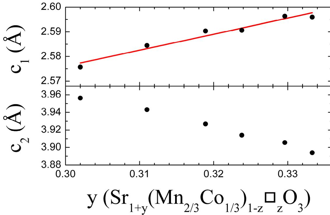
**Fig.8** Evolution of the cell parameters of the oxides  $\text{Sr}_{1+y}[(\text{Mn}_{2/3}\text{Co}_{1/3})_{1-z}\square_z]\text{O}_3$  versus  $y$
