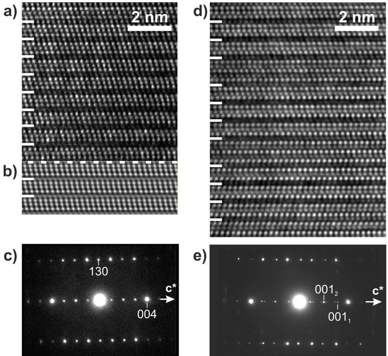
**Fig. 11:** Transmission electron microscopy observation along the [3-10] direction of two members of the  $\text{Sr}_{1+x}(\text{Mn}_{1-x}\text{Co}_x)\text{O}_{3+\delta}$  compounds. In a) HREM image, b) HREM image simulation (thickness 17.3 nm, defocus 75 nm) and c) SAED patterns for  $\gamma=2/3$ . In d) HREM image and e) SAED patterns for  $\gamma\approx 0.64$ .
