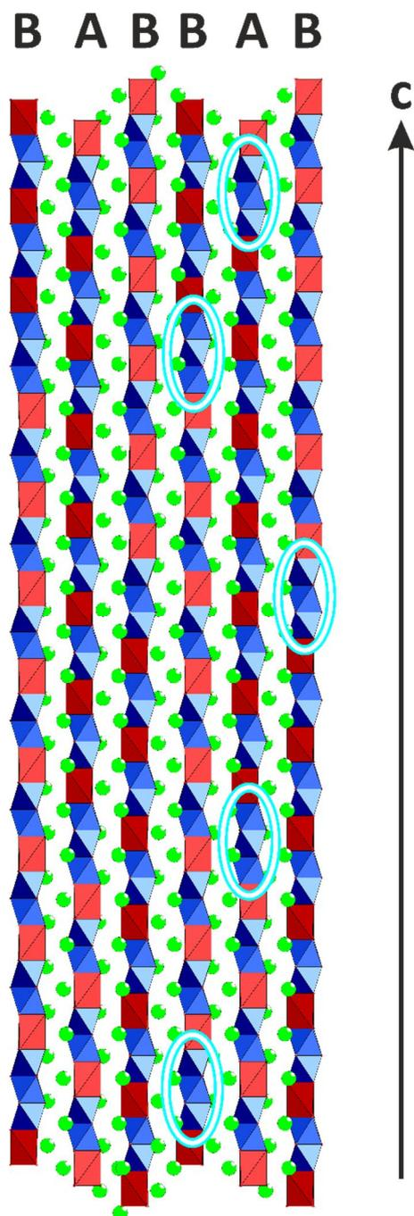
**Fig. 9:** Projection along the  $[1\ 2\ 0]$  direction of 6 prism–octahedra columns (BABBAB) depicted in the figure 6 for the crystals II. Sequences of three successive Oh are cyan circled.
