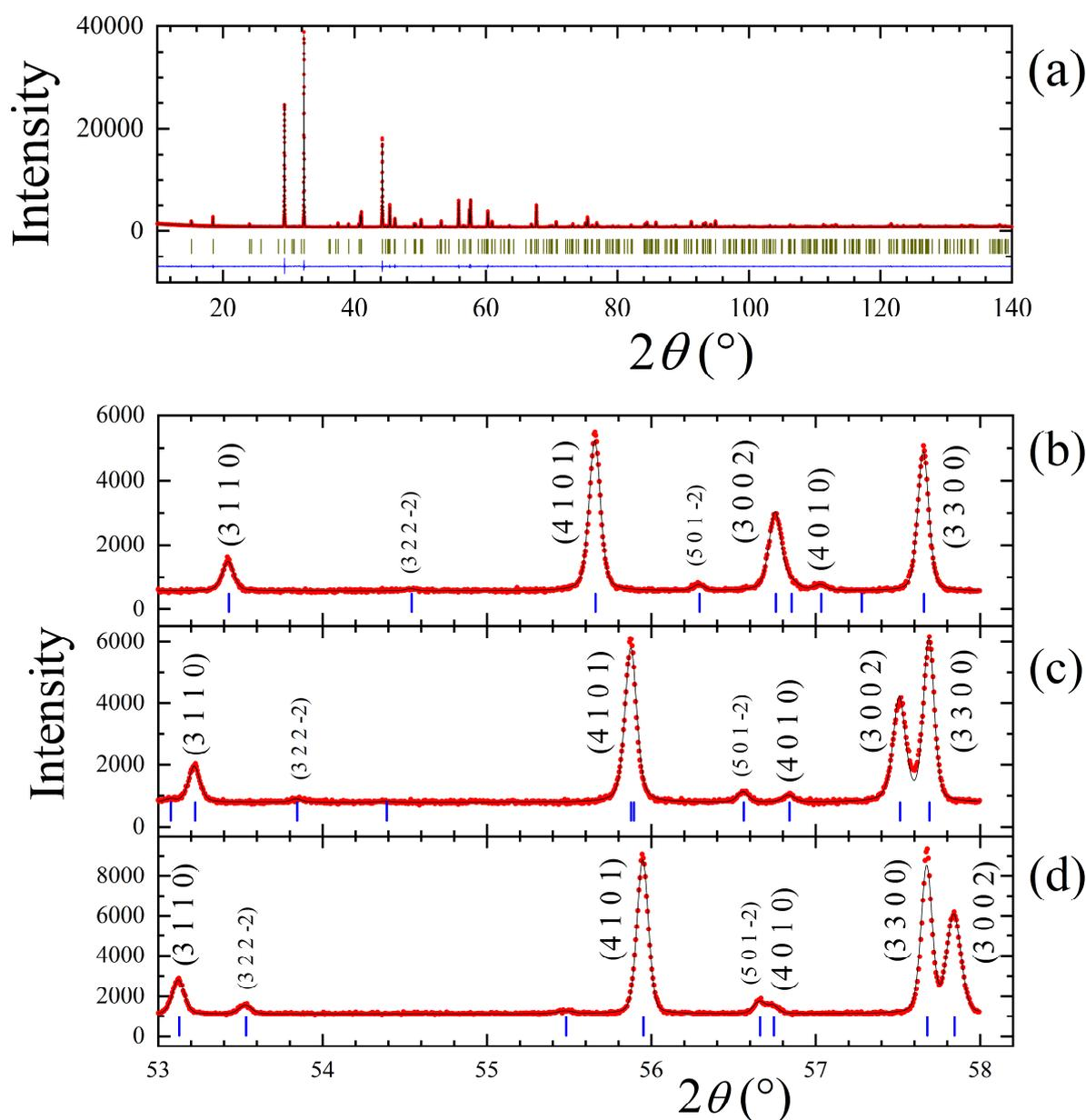
**Fig.2** Powder X-Ray diffraction pattern of  $\text{Sr}_{1+x}(\text{Mn}_{1-x}\text{Co}_x)\text{O}_{3+\delta}$  for  $x=7/20$  (a) and part of PXRD patterns showing the shifting of main and satellite reflections for  $x=2/7$  (b),  $x=7/20$  (c) and  $x=3/8$  (d).
