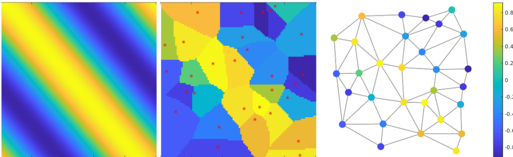
Figure 13: Sample graph in Band-Pass graph dataset. Random rotated and translated image pattern with frequency of 1, random sampled points and their watershed regions, and graph represent the connected region and average region intensity value respectively.
