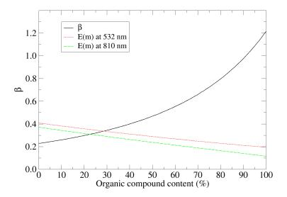
Figure 2: Relationship between the maturity coefficient  $\beta$  and absorption functions E(m) at 532 and 810 nm and the content of organic material in soot particles expressed as volume percentage.
