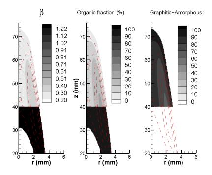
Figure B.10: Distribution of the determined maturity coefficient  $\beta$  and the corresponding organic and mature graphitic soot contents using synthetic images based on CoFlame simulation. Red dash lines represents volume fraction isovalues.
