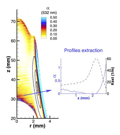
Figure 6: Contribution of soot scattering to extinction measurement at  $\lambda = 532$  nm. The black dashed lines display the iso-values of extinction coefficient at 810 nm in order to locate the soot volume fraction region. The inset presents the extracted profiles along the blue dot-dash line. The black dashed curve displays  $k_{ext}$  measured at 810 nm and the blue solid curve shows  $\alpha$  determined at 532 nm.
