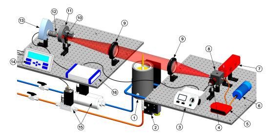
Figure 3: Schematic of the optical rig: (1) burner, (2) translation stage, (3) LED driver, (4) LED source, (5) spectrometer, (6) calibrated light source, (7) stabilized broadband light source, (8) integrating sphere, (9) achromatic lens, (10) neutral density filters, (11) spectral filter wheel, (12) camera lens, (13) Andor CCD camera, (14) mass flow readout module, (15) mass flow controllers, and (16) pulse generator.
