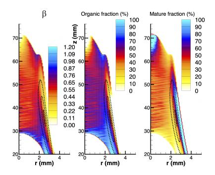
Figure 5: Retrieved distributions of the soot maturity coefficient  $\beta$  and the corresponding to organic and mature (graphitic) soot contents in the laminar coflow ethylene/air diffusion flame based on experimental measurements. The black dashed lines indicate the iso-values of extinction coefficient at 810 nm to help locate the sooting region.
