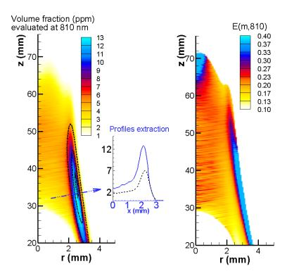
Figure 7: Distributions of the absolute E(m) at  $\lambda=810$  nm (right plot) and the corresponding soot volume fraction (left plot). Black dashed lines show the iso-values of extinction coefficient at 810 nm. The inset shows the  $f_v$  profiles along the blue dot-dash line using a constant E(m)=0.37 (black dashed line) and the spatially varying E(m) (solid blue line).
