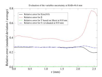
Figure E.14: Radial profiles uncertainties based on a Monte-Carlo error propagation approach at  ${\rm HAB}=46.6~{\rm mm}.$
