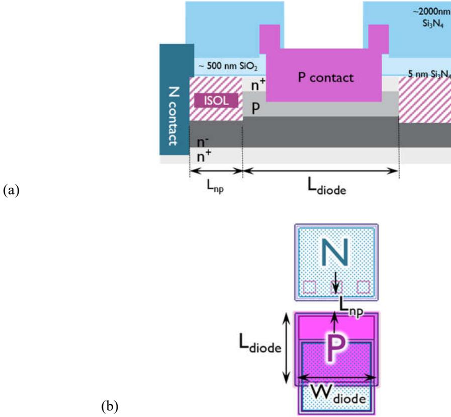
**Figure 1.** Schematic representation of the GaN-on-Si  $p^+n$ -diode under study, showing the diode in a cross-sectional view (a) and in top view (b). The diodes under study have an area of  $100 \times 112 \mu\text{m}^2$  ( $L_{\text{diode}} \times W_{\text{diode}}$ ) and there is a  $14 \mu\text{m}$  distance between the top N and P contact area ( $L_{\text{np}}$ ).
