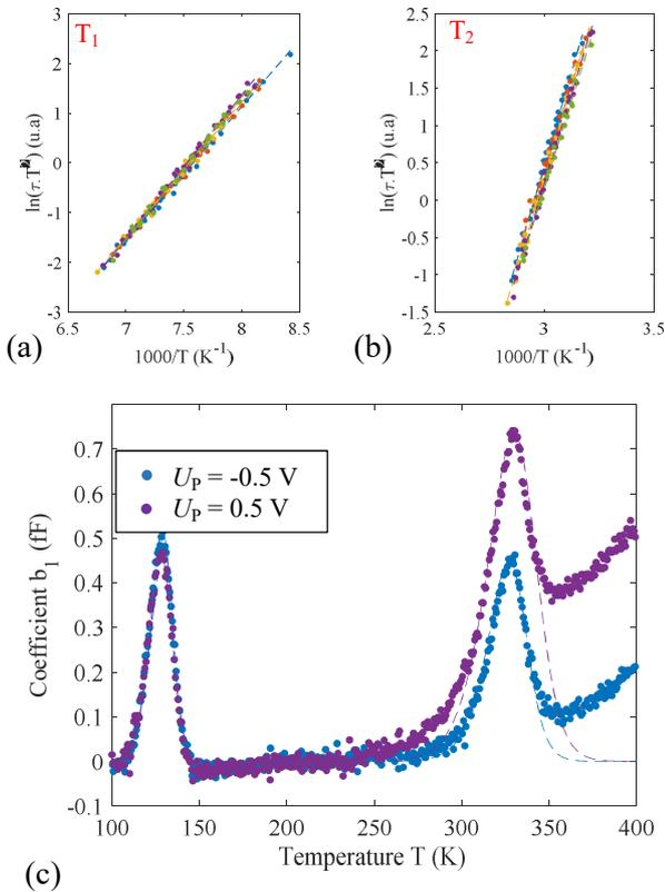
**Figure 7.** Arrhenius plots of the defect state (a) at 130 K and (b) at 330 K extracted for different values of  $U_R$  and for  $U_p = -0.5$  V. (c) DLTFs spectra at  $U_R = -5$  V for  $U_p = -0.5$  V (in blue) and  $U_p = 0.5$  V (in violet) and their fit using the extracted parameters.
