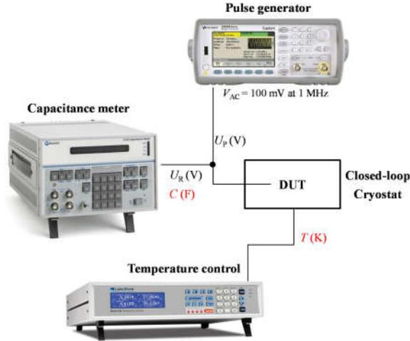
**Figure 3.** Schematic of the measurement setup composed of a capacitance meter (Boonton 7200), a pulse generator (Agilent 33500B), a temperature controller (Lakeshore Model 336) and a PhysTech FT-1230 HERA DLTS system (not shown). The sample is placed in a closed-loop He cooled cryostat.
