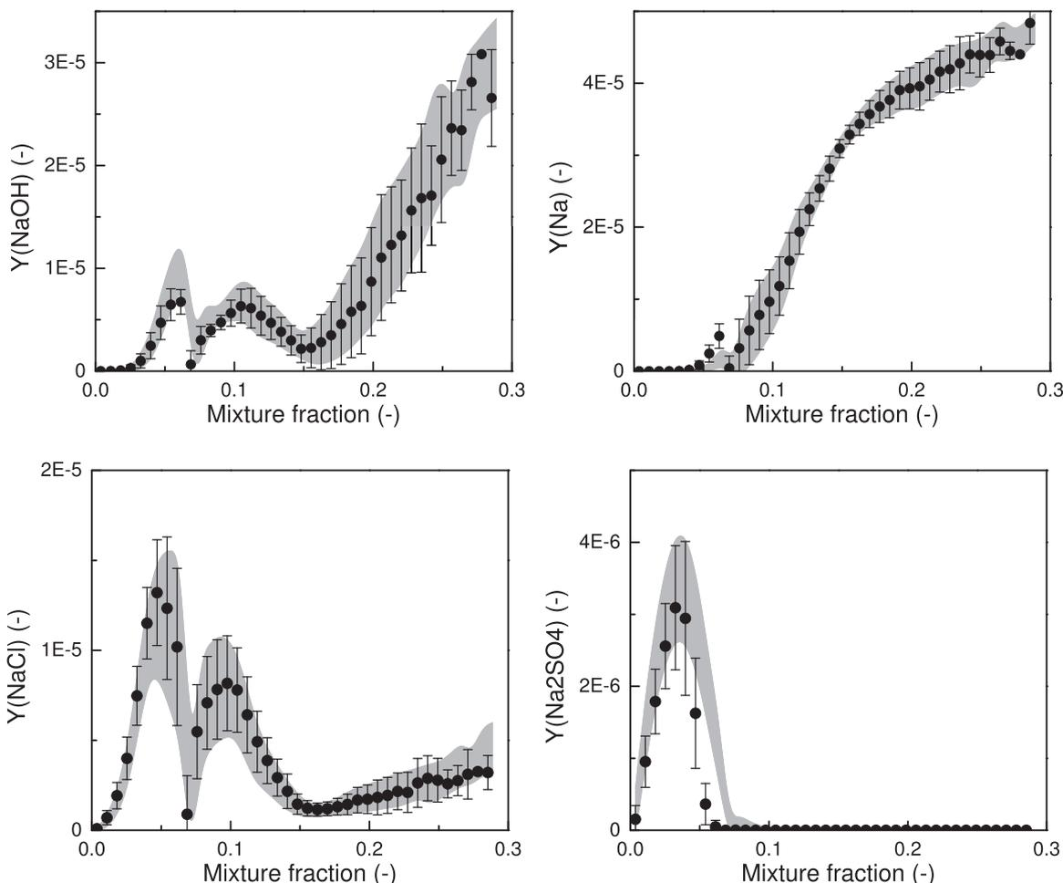
Fig. 16. Conditional mixture fraction averages at  $t = 10$  ms. NaOH, Na, NaCl and Na<sub>2</sub>SO<sub>4</sub>. Range of the conditional mean  $\pm$  fluctuation, grey bands: reference chemistry [26,42], symbols: global mechanism (Table 5).
