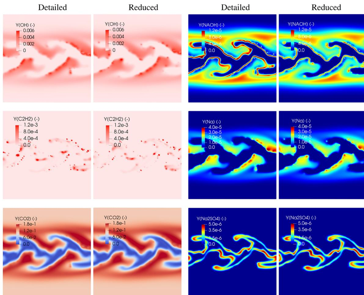
Fig. 10. Instantaneous distributions of mass fractions of OH, NaOH, C<sub>2</sub>H<sub>2</sub>, Na, CO<sub>2</sub> and Na<sub>2</sub>SO<sub>4</sub> at  $t = 10$  ms. Transverse plane  $z = 0$ . Left columns: reference mechanism [26,42]. Right columns: reduced mechanism (Table 2).
