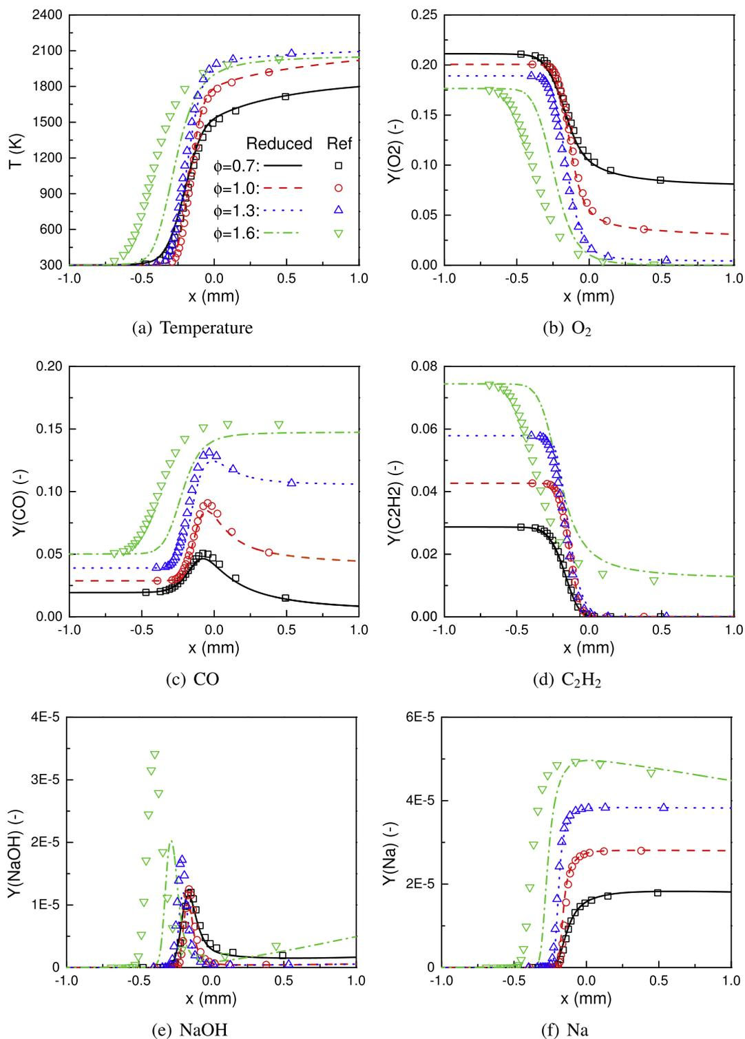
**Fig. 1.** Distribution of temperature and mass fractions in one-dimensional premixed flames. Black: Equivalence ratio  $\phi = 0.7$ . Red: 1.0. Blue: 1.3. Green: 1.6. Symbols: reference chemistry [26,42]. Lines: preliminary reduced mechanism (DRGEP, Table 2 but with original rates parameters). (For interpretation of the references to colour in this figure legend, the reader is referred to the web version of this article.)
