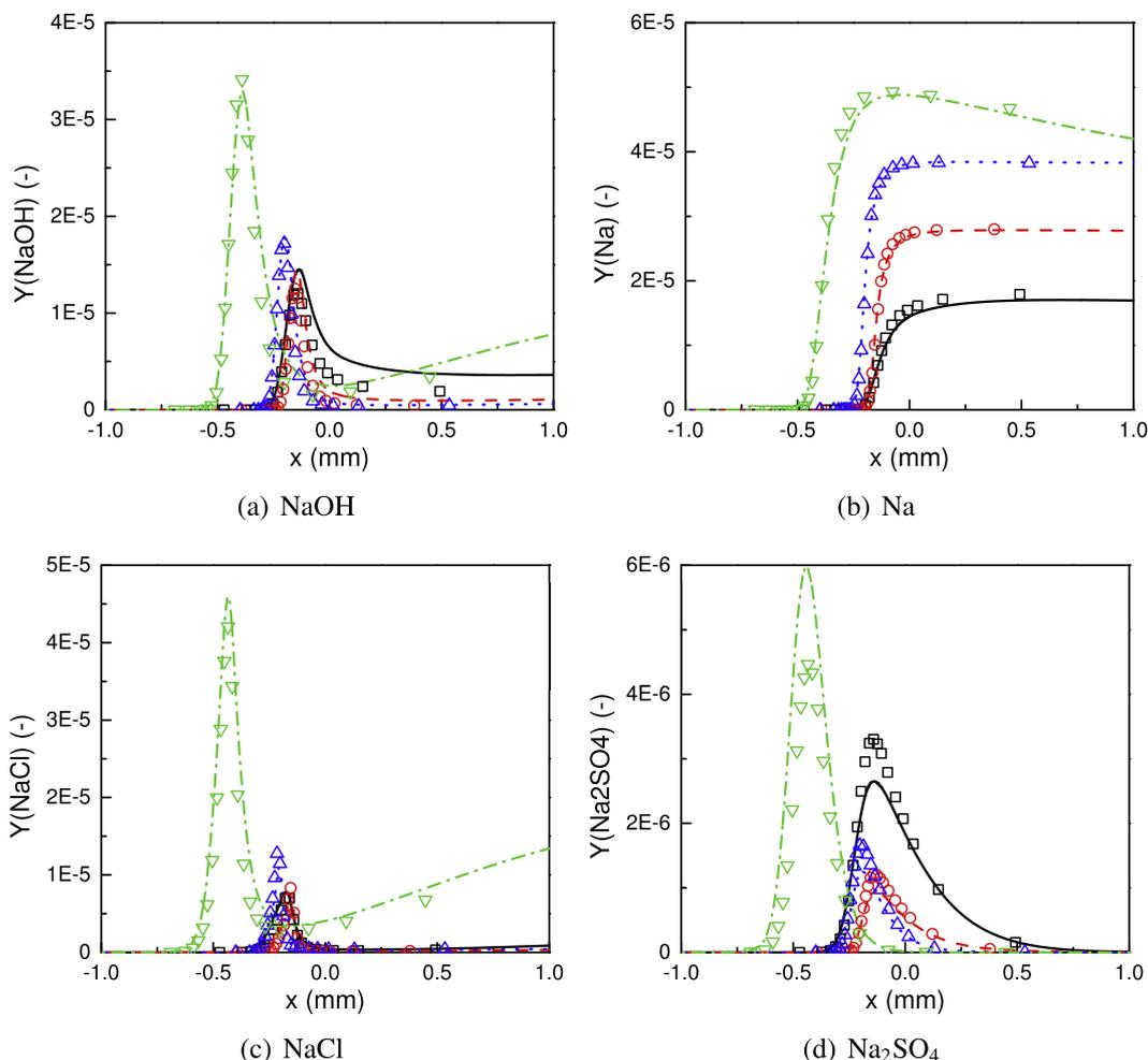
Fig. 4. Distribution of mass fractions in one-dimensional premixed flames. Black: Equivalence ratio  $\phi = 0.7$ . Red: 1.0. Blue: 1.3. Green: 1.6. Symbols: reference chemistry [26,42]. Lines: Reduced mechanism (DRGEP + Genetic Algorithm, Table 2). (For interpretation of the references to colour in this figure legend, the reader is referred to the web version of this article.)
