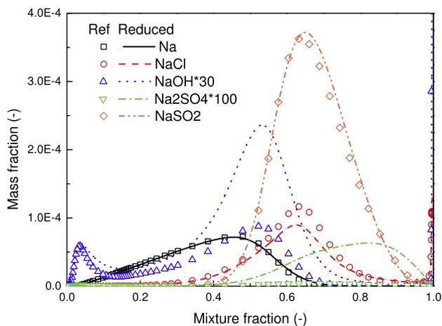
Fig. 6. Species mass fractions and temperature distributions in one-dimensional diffusion flames (strain rate  $5052 \text{ s}^{-1}$ ). Symbol: reference chemistry [26,42]. Lines: reduced chemistry (Tables 2 and 3).
