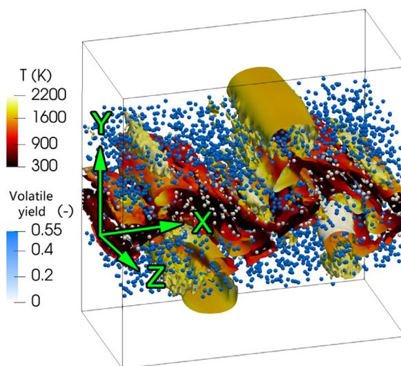
Fig. 7. Instantaneous pulverized-coal particle distribution and iso- $Q$ -criterion [63] of  $Q = 10^3 \text{ s}^{-2}$  colored by gas temperature. The coal particles are colored by the volatile yield, which denotes the ratio of the released volatile mass to the initial mass of a coal particle.
