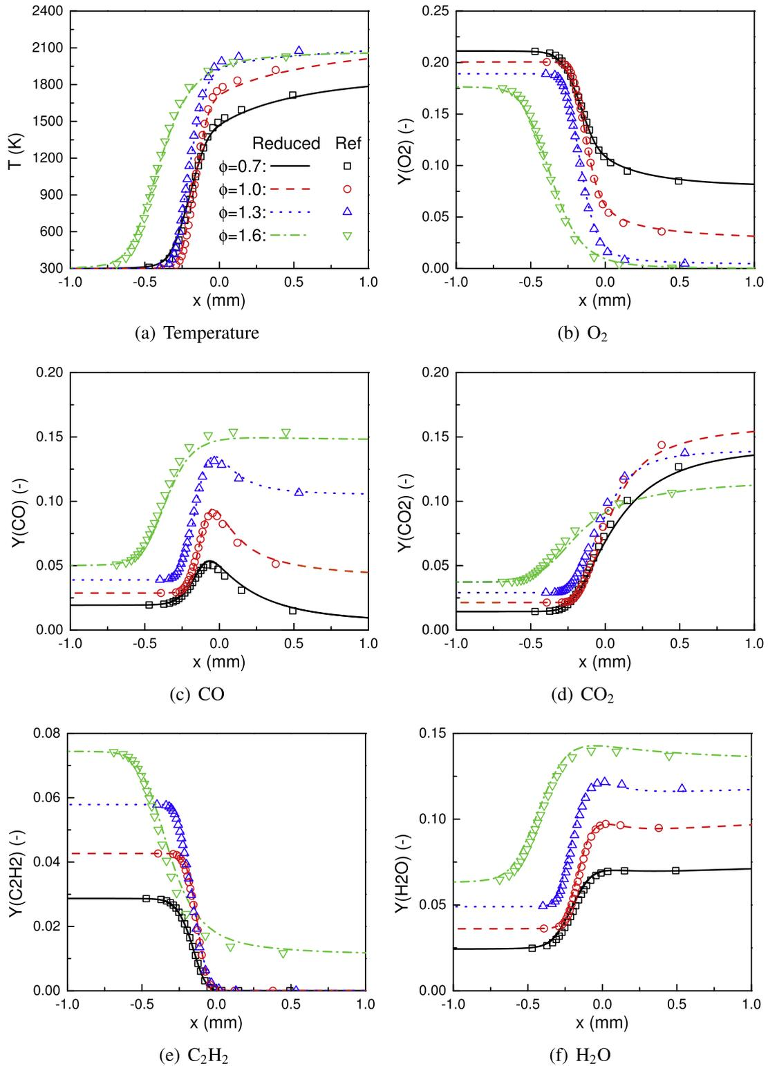
**Fig. 3.** Distribution of temperature and mass fractions in one-dimensional premixed flames. Black: Equivalence ratio  $\phi = 0.7$ . Red: 1.0. Blue: 1.3. Green: 1.6. Symbols: reference chemistry [26,42]. Lines: Reduced mechanism (DRGEP + Genetic Algorithm, Table 2). (For interpretation of the references to colour in this figure legend, the reader is referred to the web version of this article.)
