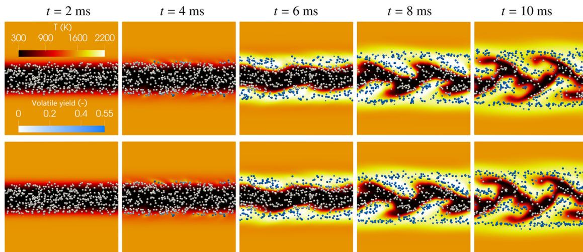
Fig. 8. Instantaneous distributions of the gas temperature and particle volatile yield at subsequent times. Transverse plane  $z = 0$  and coal particles in  $|z| \leq 100 \mu\text{m}$ . Upper: reference mechanisms [26,42]. Lower: optimized reduced mechanism (Table 2).
