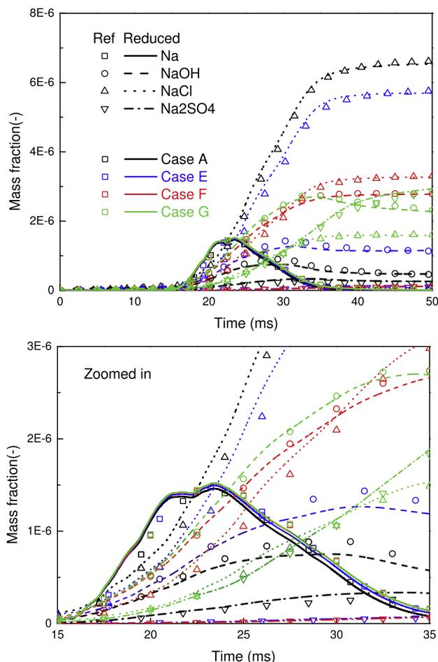
**Fig. 15.** Time evolution of averaged mass fractions. Black: Case A of Table 4. Blue: Case E. Red: Case F. Green: Case G. Symbols: reference chemistry [26,42]. Lines: reduced mechanism (Table 2). The range of time  $\in [15, 35]$  ms is zoomed in and shown on the bottom. (For interpretation of the references to colour in this figure legend, the reader is referred to the web version of this article.)
