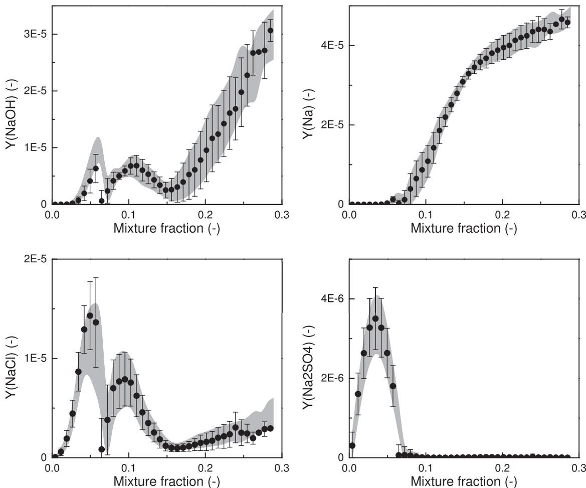
Fig. 12. Conditional mixture fraction averages at  $t = 10$  ms. NaOH, Na, NaCl and  $\text{Na}_2\text{SO}_4$ . Range of the conditional mean  $\pm$  fluctuation, grey bands: reference chemistry [26,42], symbols: reduced mechanism (Table 2).
