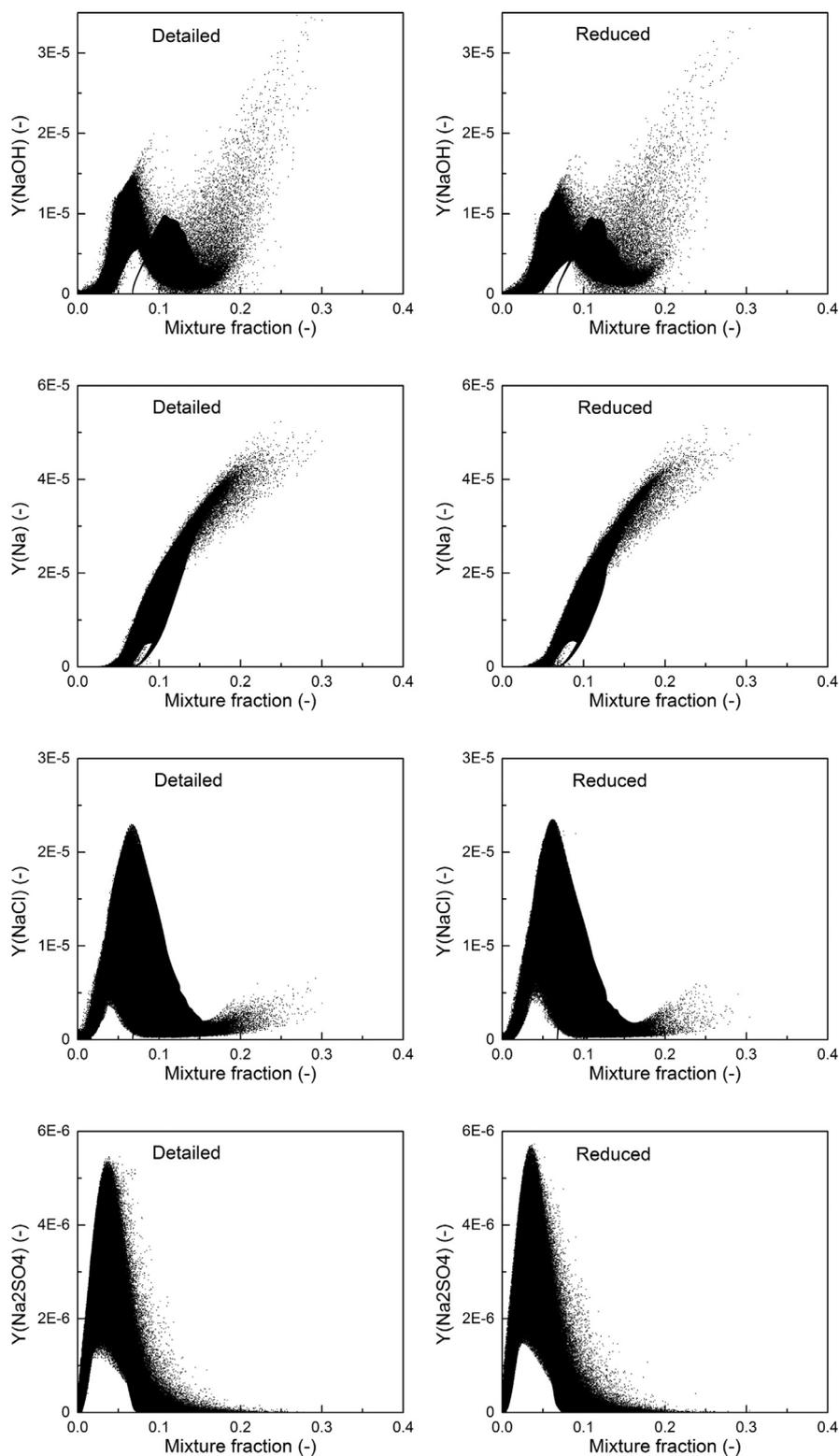
**Fig. 11.** Scatter plots of instantaneous mass fractions of NaOH, Na, NaCl, Na<sub>2</sub>SO<sub>4</sub> against mixture fraction at  $t = 10$  ms. Left: reference mechanism [26,42]. Right: reduced mechanism (Table 2).
