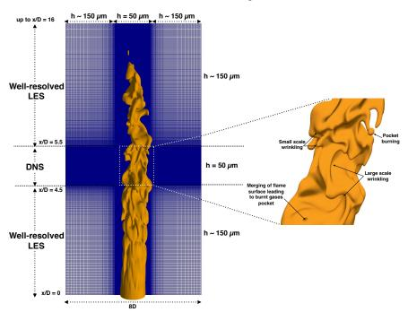
**Fig. 6** LES-DNS snapshot of the jet-flame simulation [26]. Mesh and iso-progress variable c = 0.8. *h*: resolution. Right: zoom of iso-c = 0.8 in the DNS zone (different angle view). Reprinted with permission [26].
