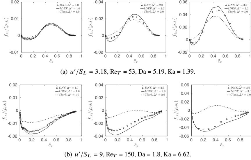
**Fig. 5** SGS convective flux in the direction normal to the mean flame front averaged in the transverse plane, plotted versus a progress variable ( $c_x = 0$  in fresh gases and  $c_x = 1$  in fully burnt gases).  $\circ$ : DNS. —: IDEF. ---: Clark model [32]. Left:  $\Delta/\delta_L = 1$ , Middle: 2, Right: 3. Reprinted with permission [31].
