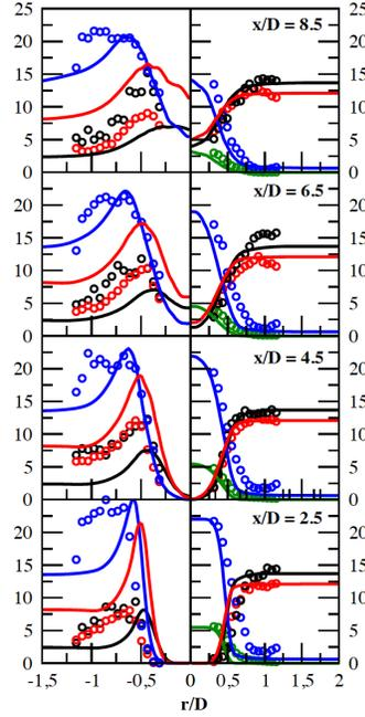
**Fig. 3** Mass fractions in %. Symbol measurements [17]. Line: LES. In each subfigure: Left: Red:  $\text{CO} \times 10$ . Black:  $\text{H}_2 \times 100$ . Blue:  $\text{OH} \times 75$ . Right: Blue:  $\text{O}_2$ . Green:  $\text{CH}_4$ . Red:  $\text{H}_2\text{O}$ . Black:  $\text{CO}_2$ . Reprinted with permission [26].
