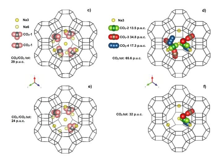
Figure 3. Structures of the zeolite samples under different conditions: (a) Na-X-RT, (b) Na-Y-RT, (c) Na-X- $CO_2$  (after CO<sub>2</sub> adsorption), (d) Na-Y- $CO_2$  (after CO<sub>2</sub> adsorption), (e) Na-X-AP (after CO<sub>2</sub> desorption), and (f) Na-Y-AP (after CO<sub>2</sub> desorption); a, b: the Na sites are drawn according to their occupancy factors; c, d, e, f: only the Na sites in the supercage are shown. Water molecules are not shown for sake of clarity.
