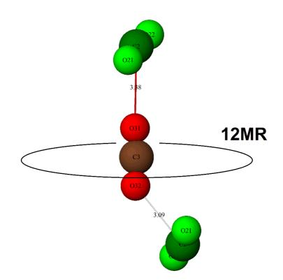
Figure 7. Interactions among CO<sub>2</sub>-2 and CO<sub>2</sub>-3 molecules in neighboring supercages in Na-Y-*CO*<sub>2</sub> sample.
