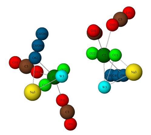
Figure 6. Possible distribution of  $CO_2$  molecules, Na cations and W3 molecule in the supercage of the Na-Y-*CO*<sub>2</sub> sample (only Na3 and W3 bonded to the clusters are drawn). The labels C2, O21 and O22 represent the CO<sub>2</sub>-2 molecule, C3, O31 and O32 the CO<sub>2</sub>-3 molecule and C4, O41 and O42 the CO<sub>2</sub>-4 one.
