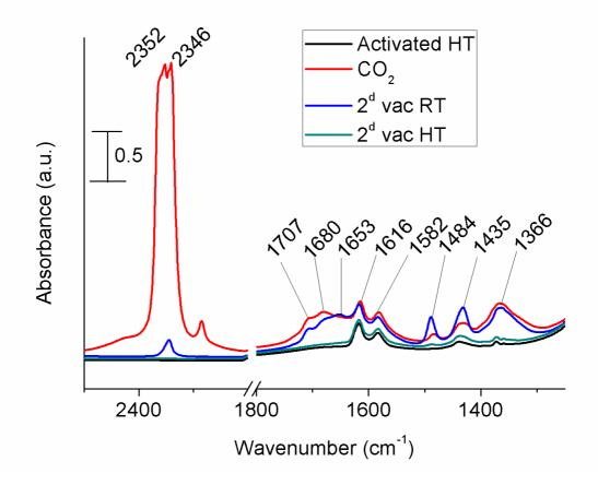
Figure 8. FTIR spectra of nanosized Na-X zeolite activated at 250 °C (black), after adsorption of 0.01 Bar CO<sub>2</sub> (red), under secondary vacuum ( $\sim 5 \cdot 10^{-9}$  Bar) at room temperature (blue), and under secondary vacuum ( $\sim 5 \cdot 10^{-9}$  Bar) and at 250 °C (green).
