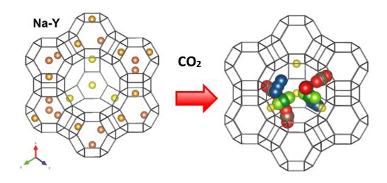
Nano Na-X and Na-Y before and after  $\rm CO_2$  adsorption
