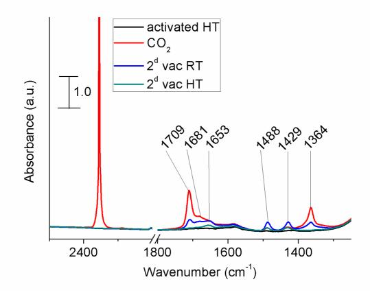
Figure 9. FTIR spectra of nanosized Na-Y zeolite under activation at 250 °C (black), after adsorption of 0.01 Bar CO<sub>2</sub> (red), under secondary vacuum ( $\sim 5 \cdot 10^{-9}$  Bar) at room temperature (blue), and under secondary vacuum ( $\sim 5 \cdot 10^{-9}$  Bar) and activation at 250 °C (green).
