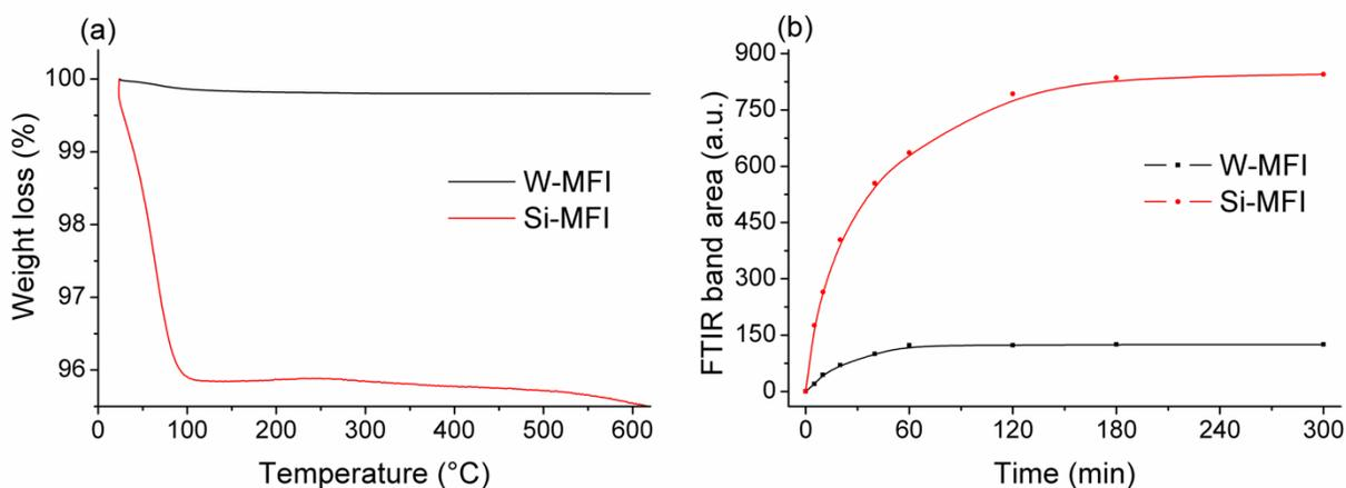
**Figure 2.** (a) Water content in calcined W-MFI (black) and Si-MFI (red) powder samples stored at 70% relative humidity (RH) after 7 days measured by TG and (b) water adsorption on activated W-MFI-1600 (black) and Si-MFI-1600 (red) films exposed to 100 ppm of water for 300 minutes monitored by *operando* FTIR spectroscopy (band area at 1600 cm<sup>-1</sup>).
