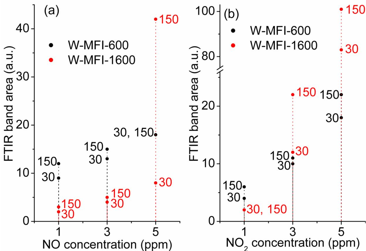
**Figure 3.** Responses of activated zeolite films W-MFI-600 (black) and W-MFI-1600 (red) exposed to (a) NO and (b) NO<sub>2</sub> gas (concentrations 1-5 ppm) in the presence of 100 ppm of water monitored by *operando* FTIR spectroscopy after 30 and 150 seconds.
