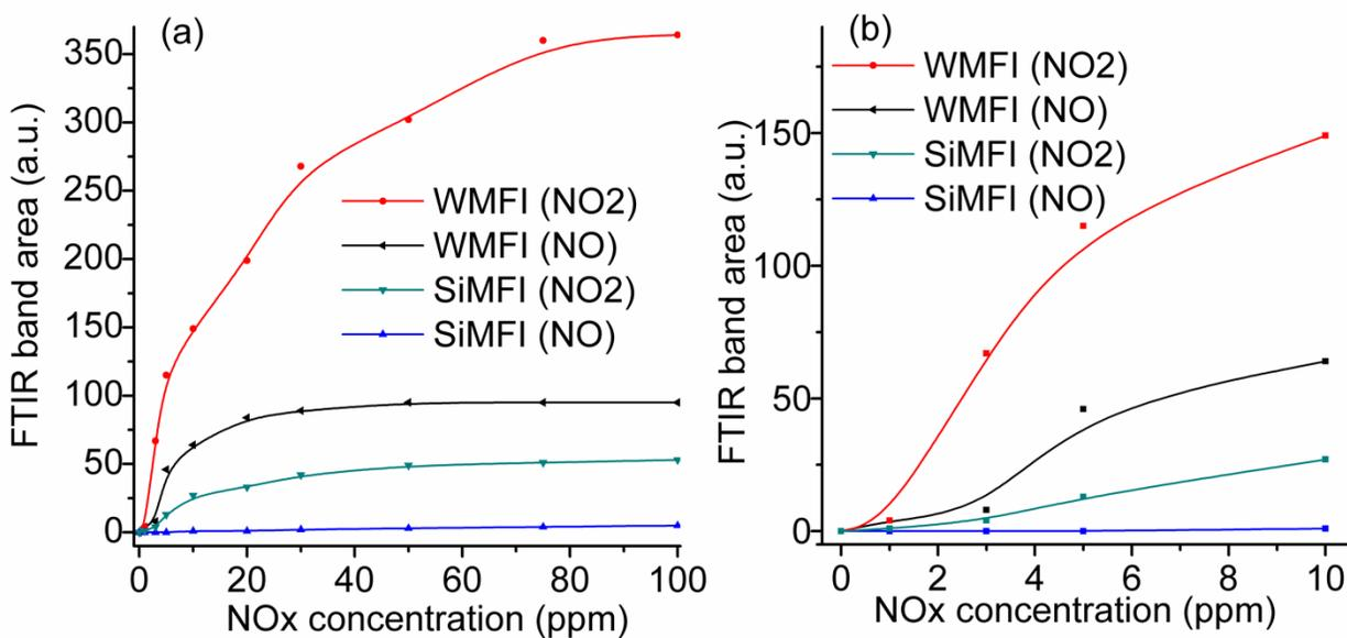
**Figure 4.** Detection of NO with W-MFI-1600 (black) and Si-MFI-1600 (blue), and NO<sub>2</sub> with W-MFI-1600 (red) and Si-MFI-1600 (green) films; IR band areas (1650 - 1480 cm<sup>-1</sup>) are measured at concentrations (a) 1-100 ppm and (b) 1-10 ppm NO and NO<sub>2</sub>.
