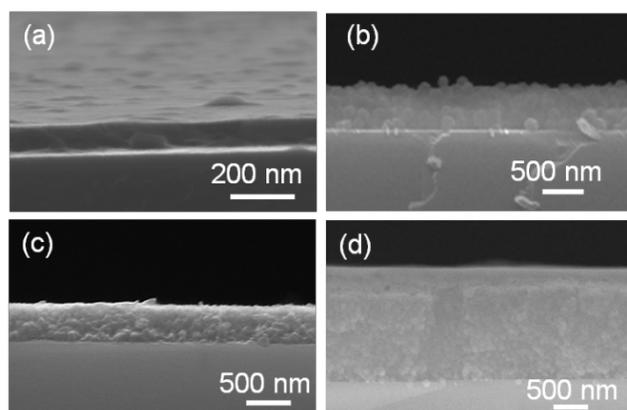
**Figure 1.** FE-SEM side-view images of (a) as-deposited PVP binder layer (100 nm), (b) calcined Si-MFI film (600 nm), (c) calcined W-MFI-600 film (600 nm) and (d) calcined W-MFI-1600 films (1600 nm).
