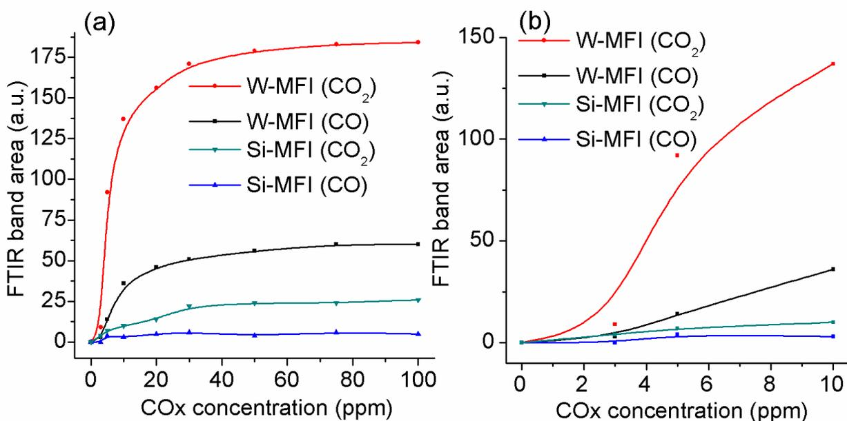
**Figure 5.** Detection of CO with W-MFI-1600 (black) and Si-MFI-1600 (blue) films and CO<sub>2</sub> with W-MFI-1600 (red) and Si-MFI-1600 (green) films following the evolution of the band areas corresponding to chemisorbed and physisorbed carbonates: (a) 3-100 ppm and (b) 3-20 ppm CO and CO<sub>2</sub>, respectively.
