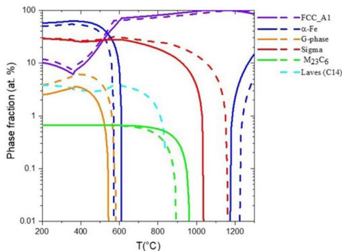
**Fig. 2.** Predictive equilibrium phase fractions calculation as function of temperature. Dash lines correspond to phase fraction for Mo-bearing steels and continuous lines to phase fraction for Mo-free steels. [20]. (For interpretation of the references to colour in this figure legend, the reader is referred to the web version of this article.)
