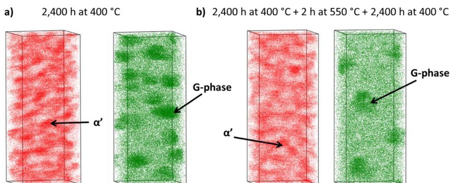
**Fig. 3.** Cr atoms distributions (red) and Ni+Si+Mn+Mo atoms distributions (green) obtained by APT in ferrite of alloy G-400 (a) after 2400 h at 400 °C and (b) after 2400 h at 400 °C + 2 h at 550 °C + 2400 h at 400 °C.  $V = 20 \times 20 \times 50 \text{ nm}^3$ . (For interpretation of the references to colour in this figure legend, the reader is referred to the web version of this article.)
