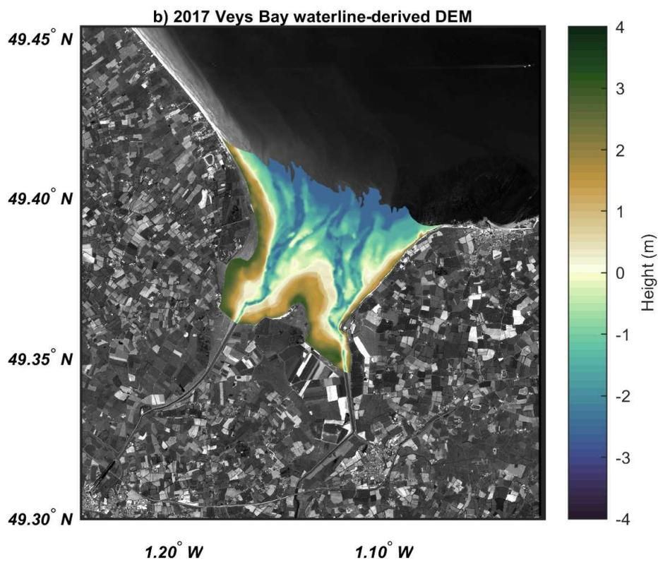
Figure 13. Veys Bay waterline-derived DEMs for: (a) 2016; (b) 2017; and (c) 2018.
