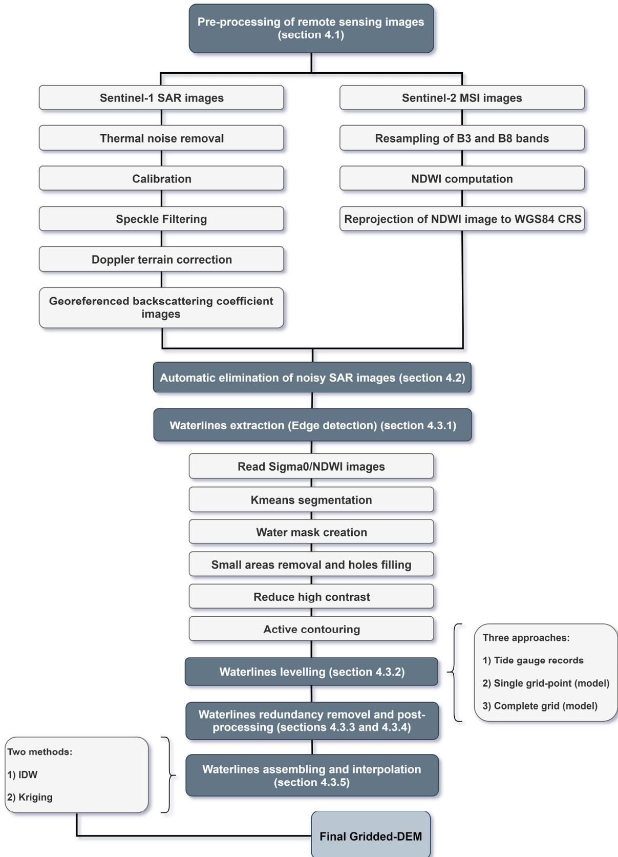
**Figure 3.** A step by step overview of the methods used in this study to generate Digital Elevation Models (DEMs) using the waterline method along with the corresponding sections.
