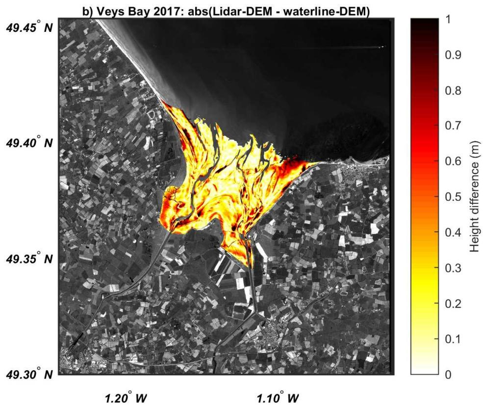
**Figure 10.** Absolute difference between a) Arcachon lidar-derived DEM (2013) and the 2016 waterline-derived DEM; b) Veys Bay lidar-derived DEM (2017) and the 2017 waterline-derived DEM.
