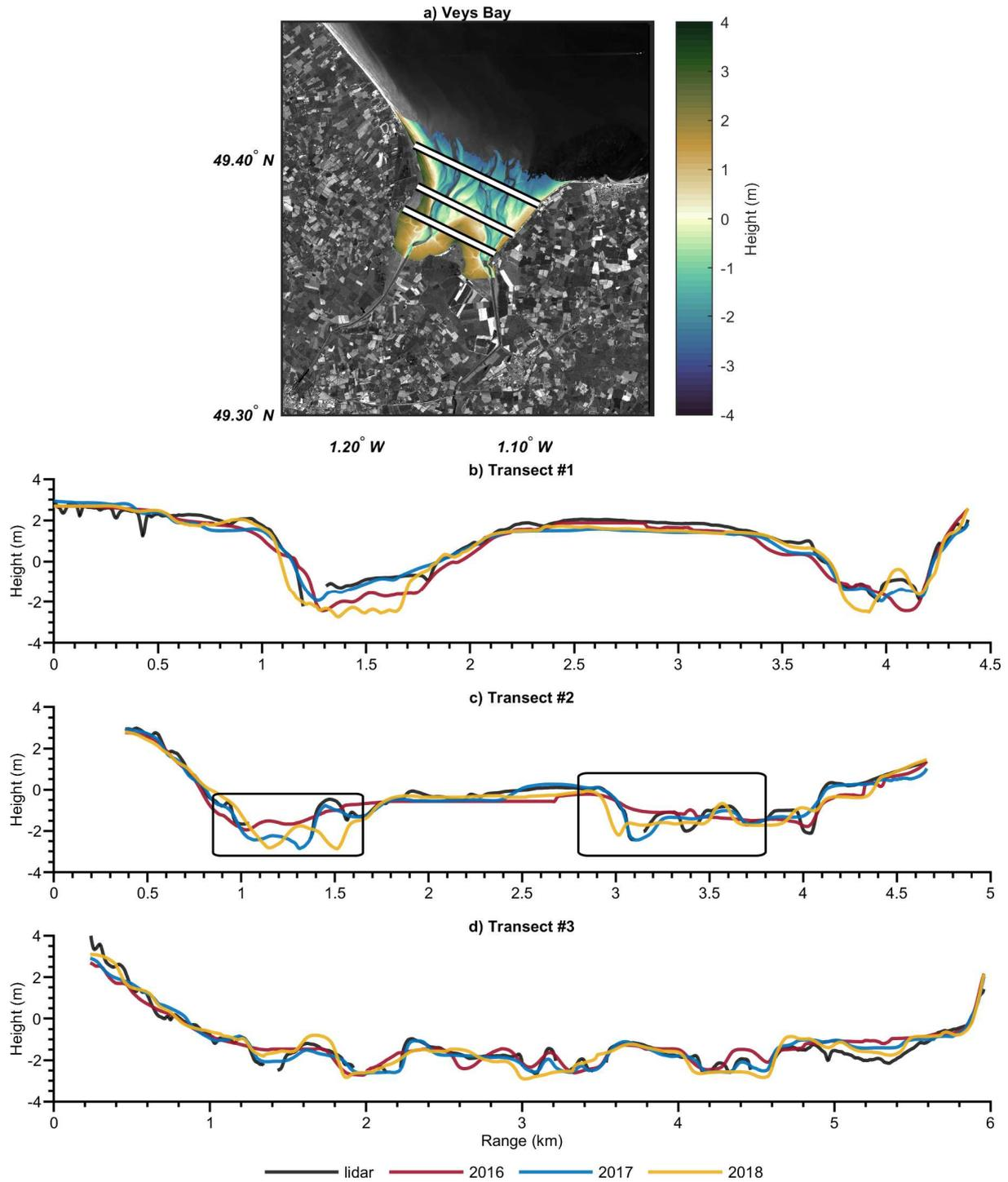
**Figure 17.** Topography profiles comparison between the lidar-derived DEM and the 2016, 2017, and 2018 waterline-derived DEMs over the Bay of Veys along three transects (#1 lower transect; #2 middle transect; #3 upper transect).
