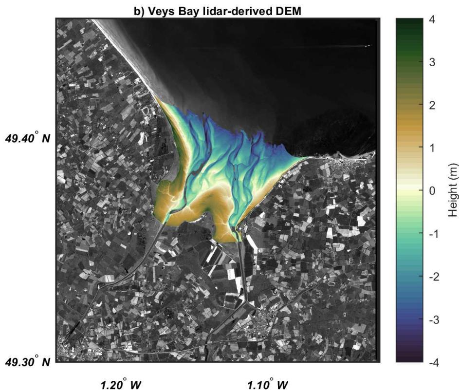
**Figure 2.** Lidar-derived DEMs used for validation for the (a) Arcachon Bay (extracted from the RGE ALTI® product provided by the national institute for geography and forest information (IGN)) and (b) the Bay of Veys (extracted from the NHDF (lidar Normandie Hauts-De-France) 2016-2017 V.20180501 product provided by the SHOM (Shom-ROLNP, 2018)). Heights are referenced to the French Reference System NGF/IGN69 datum.
