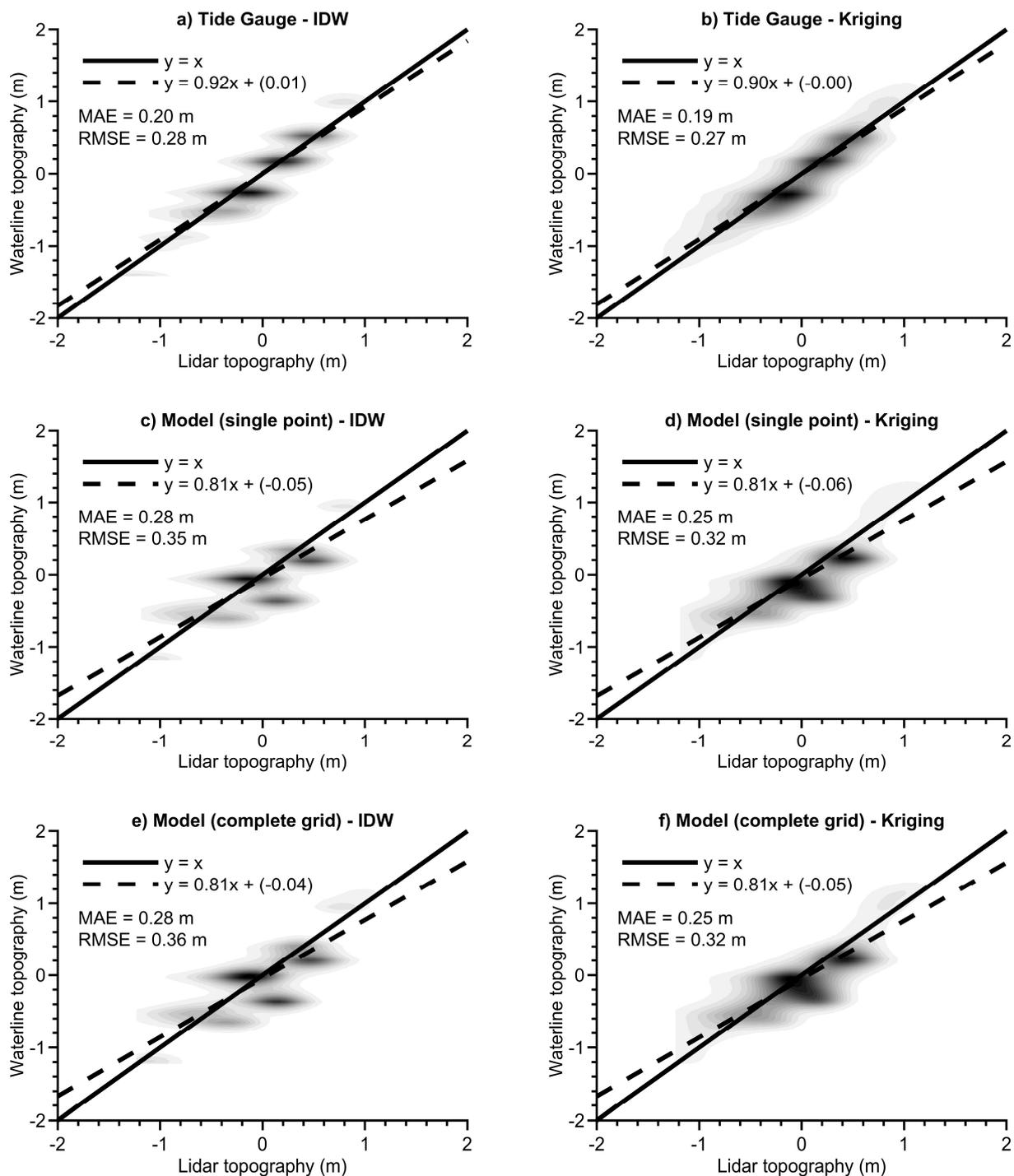
**Figure 8.** Comparisons between the lidar-derived DEM and the 2016 waterline-derived DEMs for the Arcachon Bay generated using: (a) IDW interpolation and tide gauge levelling; (b) kriging interpolation and tide gauge levelling; (c) IDW interpolation and single point model levelling; (d) kriging interpolation and single point model levelling; (e) IDW interpolation and complete grid model levelling; (f) kriging interpolation and complete grid model levelling.
