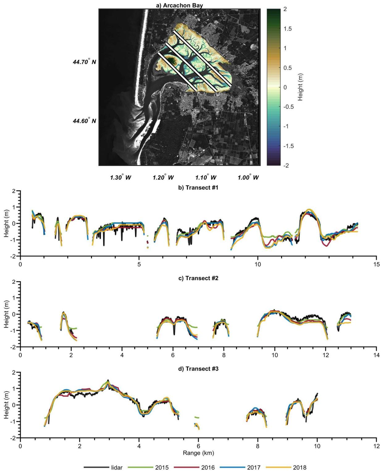
**Figure 16.** Topography profiles comparison between the lidar-derived DEM and the 2015, 2016, 2017, and 2018 waterline-derived DEMs over the Arcachon Bay along three transects (#1 upper transect; #2 middle transect; #3 lower transect).
