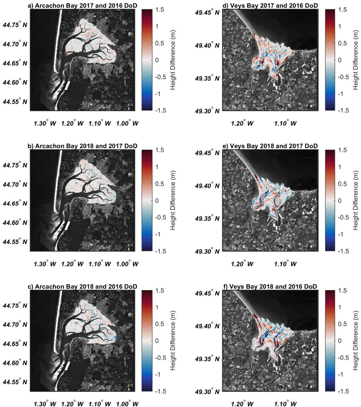
**Figure 14.** Intertidal flats DEM of Difference (DoD) maps for the Arcachon Bay between a) 2017-2016; b) 2018-2017; c) 2018-2016; and for the Veys Bay between d) 2017-2016; e) 2018-2017; f) 2018-2016.
