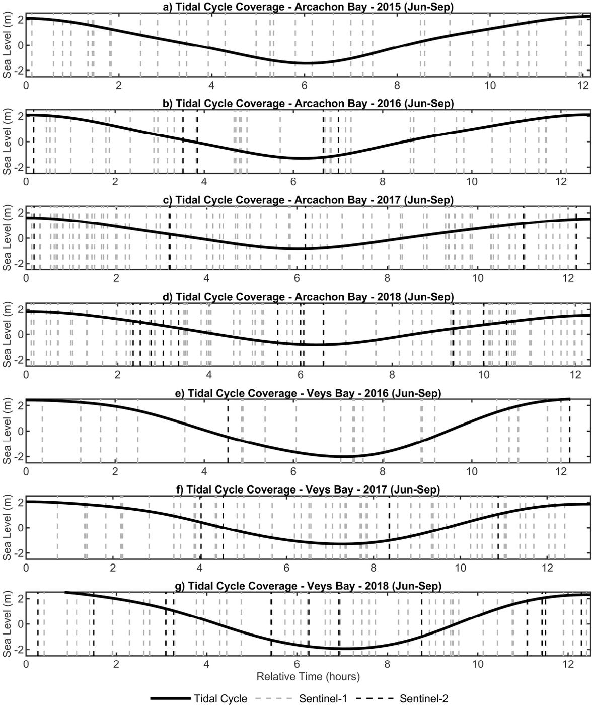
**Figure 15.** The evolution of the tidal coverage provided by Sentinel-1 and Sentinel-2 for the June-September period between 2015 and 2018 in the Arcachon and Veys Bays.
