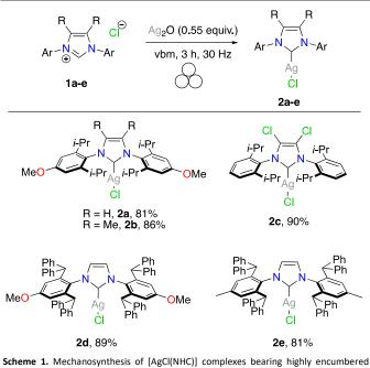
Scheme 1. Mechanosynthesis of [AgCl(NHC)] complexes bearing highly encumbered NHC ligands
