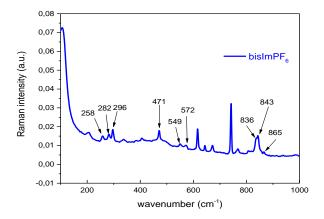
**Figure 8.** Experimental Raman vibrational spectra of bisImPF<sub>6</sub> in the frequency range 300–1000 cm<sup>-1</sup>.
