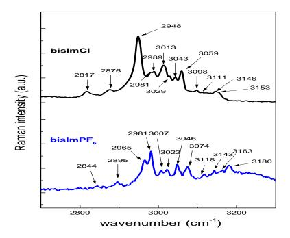
**Figure 6.** Experimental Raman vibrational spectra of bisImCl and bisImPF<sub>6</sub>in the frequency range  $2600-3500 \text{ cm}^{-1}$ .
