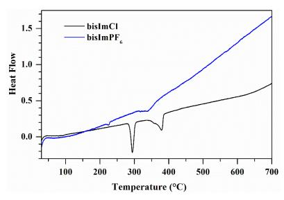
**Figure 9.** Heat flow (DTA) curves for the investigated bisImCl and bisImPF<sub>6</sub>
