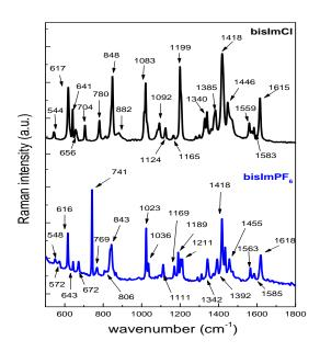
**Figure 7.** Experimental Raman vibrational spectra of bisImCl and bisImPF<sub>6</sub>in the frequency range 500–1800 cm<sup>-1</sup>.
