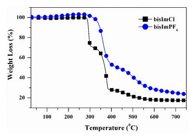
**Figure 10.** Thermal gravimetric analysis (TGA) for the investigated bisImCl and bisImPF<sub>6</sub>DILs.
