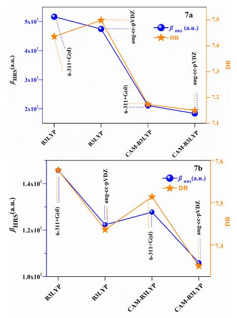
Figure 11.  $\beta_{HRS}$  and DR for bisImCl (7a) and bisImPF<sub>6</sub> (7b) obtained at different levels theory.
