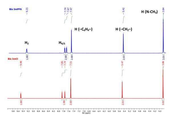
**Figure 5.**  $^{1}$ H-NMR spectra of bisImCl and bisImPF<sub>6</sub> in DMSO- $d_6$ .
