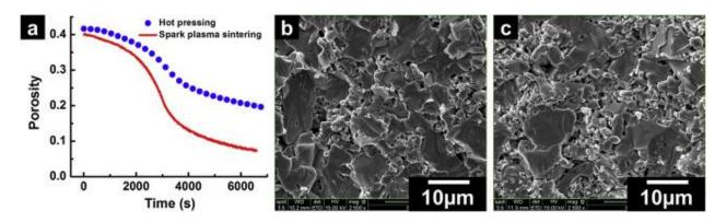
Fig. 2. (a) Porosity variation of ZrN powder densified (60 MPa and 10 °C/min) by SPS (1100 °C) and HP (1200 °C); images of the fractured surface of samples densified by (b) SPS at 1100 °C and (c) HP at 1200 °C.
