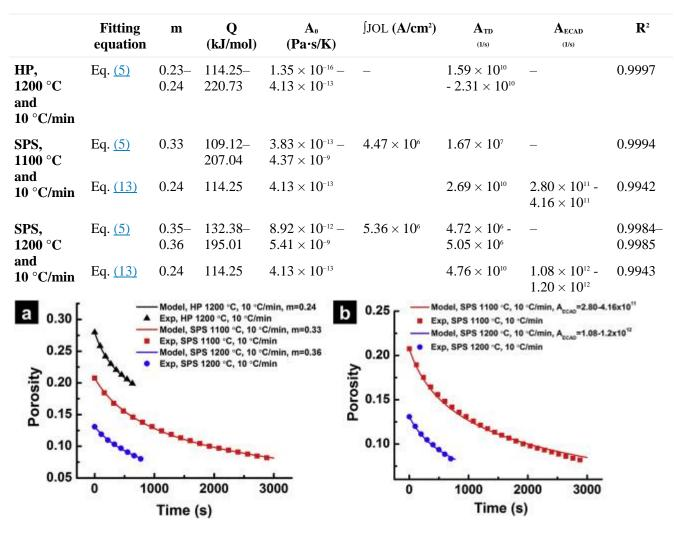
Table 3. Summary of the fitting parameters for HP and SPS of ZrN. R2 is the correlation coefficient.
