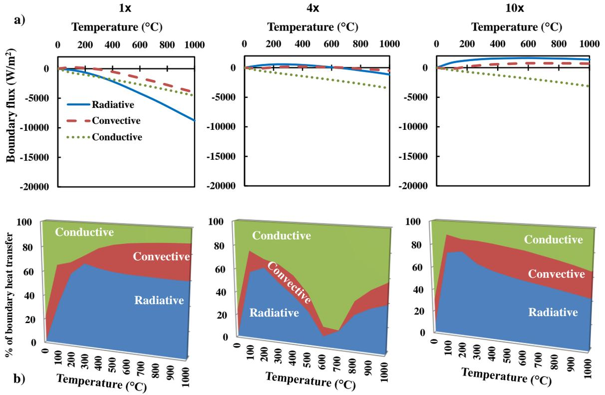
Figure 9 a) Boundary cooling fluxes curves and b) fluxes diagrams, for 1x, 4x and 10x hybrid heating configurations.
