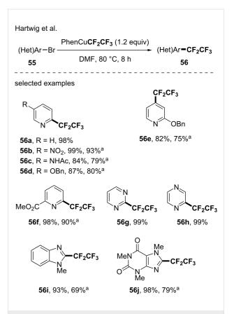
**Scheme 15:** Pentafluoroethylation of (hetero)aryl bromides using the (Phen)CuCF<sub>2</sub>CF<sub>3</sub> complex. <sup>19</sup>F NMR yields were determined using 4-trifluoromethoxyanisole as the internal standard. <sup>a</sup>Isolated yields.
