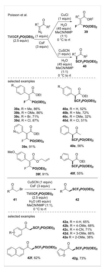
**Scheme 10:** Synthesis of (diethylphosphono)difluoromethylthiolated molecules using in situ-generated CuCF<sub>2</sub>PO(OEt)<sub>2</sub> species. Phen: 1.10-phenanthroline.
