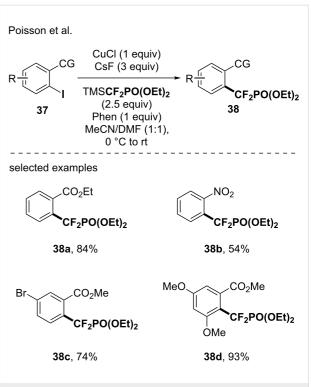
**Scheme 9:** Synthesis of difluoromethylphosphonate-containing molecules using in situ-generated  $CuCF_2PO(OEt)_2$  species by an Ullman cross-coupling. CG = coordinating group.
