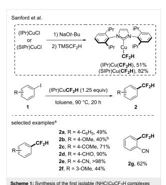
from TMSCF<sub>2</sub>H and their application for the synthesis of diffuoromethylated arenes from aryl iodides. <sup>a</sup>Yields were determined by <sup>19</sup>F NMR with fluorobenzene as the internal standard. <sup>b</sup>Reaction carried out at 120 °C.
