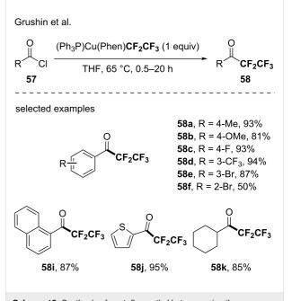
**Scheme 16:** Synthesis of pentafluoroethyl ketones using the (Ph<sub>3</sub>P)Cu(phen)CF<sub>2</sub>CF<sub>3</sub> reagent. <sup>19</sup>F NMR yields were given using 1,3-bis(trifluoromethyl)benzene as the internal standard.
