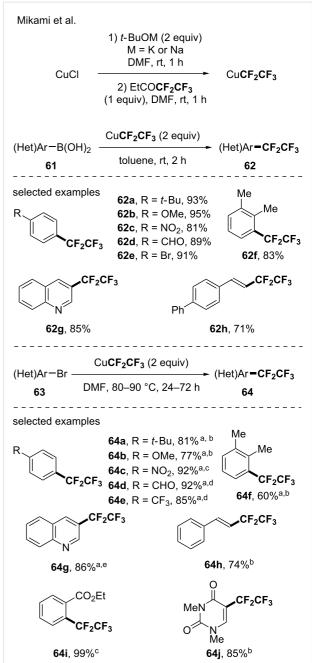
**Scheme 18:** Pentafluoroethylation of arylboronic acids and (hetero)aryl bromides via the in situ-generated CuCF<sub>2</sub>CF<sub>3</sub> species from ethyl pentafluoropropionate and CuCl. <sup>a</sup>Yields were determined by <sup>19</sup>F NMR using benzotrifluoride (BTF) or trifluoromethoxybenzene as internal standards. <sup>b</sup>90 °C, 72 h. <sup>c</sup>80 °C, 24 h. <sup>d</sup>80 °C, 48 h. <sup>e</sup>90 °C, 48 h.
