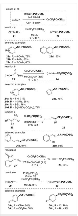
**Scheme 7:** Synthesis of difluoromethylphosphonate-containing molecules using the in situ-generated CuCF<sub>2</sub>PO(OEt)<sub>2</sub> species.
