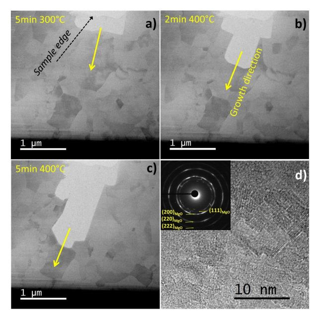
**Figure2:** STEM-BF images showing the growth of MgO inside the UFG Mg at low partial pressure of  $O_2$  and  $H_2$  (below  $10^{-5}$  Pa) (a) after 5min at 300°C, (b) after 2min at 400°C and (c) after 5min at 400°C. (d) HRTEM image taken in the oxidized region showing the nanoscaled structure of the MgO oxide, confirmed by the SAED (inset)
