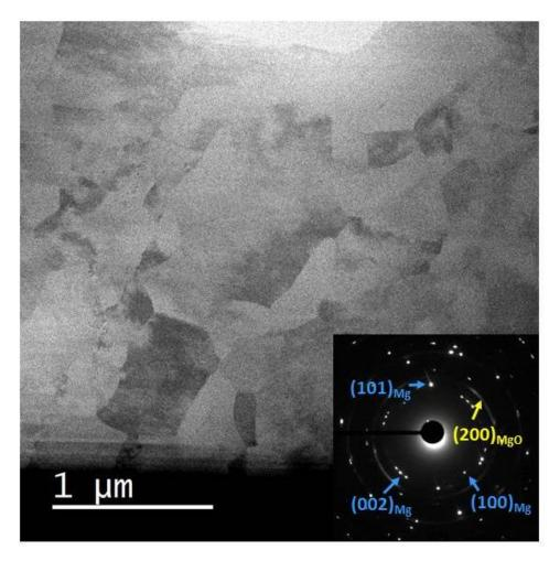
**Figure1:** STEM-BF image showing the ultrafine grain structure with large fraction of GBs. Corresponding SAED pattern (aperture size  $1.6 \mu m$ ) where spots are indexed with hcp Mg reflections and the diffuse rings are attributed to nanoscaled MgO particles on the foil surface.
