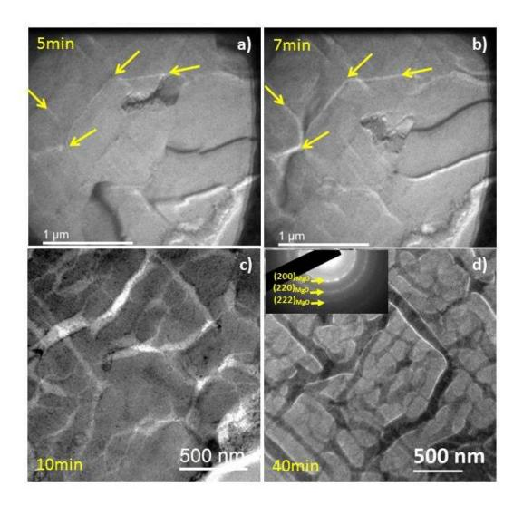
**Figure3:** TEM-BF images showing the growth of MgO along GBs (arrowed) in the UFG Mg under  $10^5$  Pa of H<sub>2</sub> and 10 Pa of O<sub>2</sub>, after 5min (a), 7min (b) and 10min (c) at 400°C. STEM-HAADF image after 40min at 400°C and SAED pattern recorded in the oxide (inset) (d)
