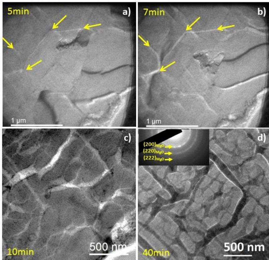
**Figure3:** TEM-BF images showing the growth of MgO along GBs (arrowed) in the UFG Mg under  $10^5$  Pa of  $H_2$  and 10 Pa of  $O_2$ , after 5min (a), 7min (b) and 10min (c) at 400°C. STEM-HAADF image after 40min at 400°C and SAED pattern recorded in the oxide (inset) (d)
