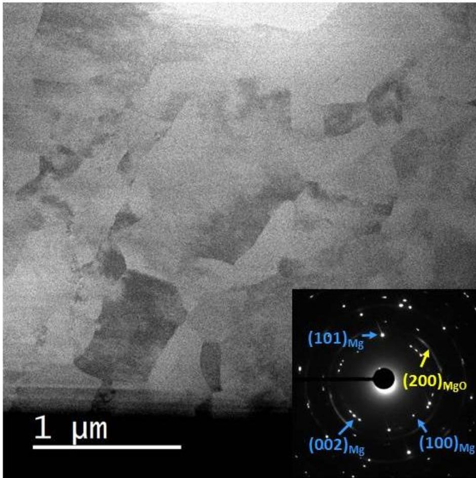
**Figure1:** STEM-BF image showing the ultrafine grain structure with large fraction of GBs. Corresponding SAED pattern (aperture size  $1.6\mu\text{m}$ ) where spots are indexed with hcp Mg reflections and the diffuse rings are attributed to nanoscaled MgO particles on the foil surface.
