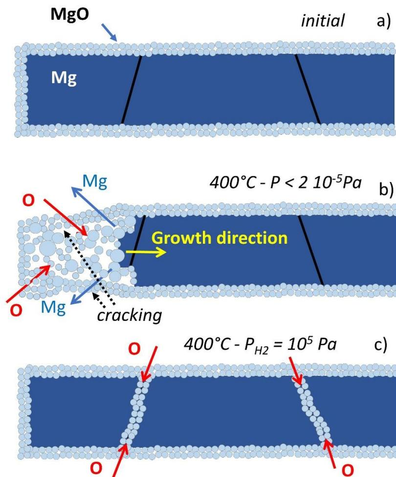
**Figure 4:** Schematic representation of the evolution of the TEM lamellae during the in-situ experiment. (a) initial state with a thin oxide layer on the surface, (b) oxidation under vacuum conditions, (c) oxidation under a high partial pressure of  $H_2$ .
