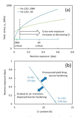
**Figure 6.** (a) Schematic representation of the cross-over from dispersed-barrier hardening (DBH) dominance to source hardening (SH) dominance for Fe-12Cr. (b) The mapping of the dominance regions of DBH and SH as function of Cr content and neutron exposure.
