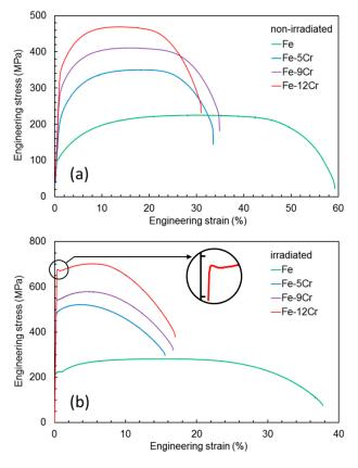
**Figure 1.** Measured engineering stress-strain curves. (a) Unirradiated and (b) irradiated conditions of the same alloys (0.2 displacements per atom (dpa) for Fe and 0.6 dpa for Fe-Cr alloys).
