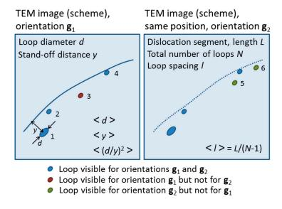
**Figure 5.** Schematic view of a dislocation segment and loops in a TEM image. <>> denotes arithmetic average.
