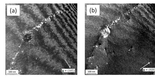
**Figure 3.** TEM weak-beam dark-field images of a dislocation decorated with loops for the Fe-12Cr alloy that was irradiated to 0.6 dpa. (a) Diffraction vector  $\mathbf{g} = (10\overline{1})$ ; (b) same detail,  $\mathbf{g} = (020)$ .
