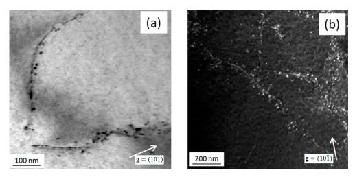
**Figure 4.** (a) TEM bright field image of the 0.6 dpa Fe-9Cr alloy and (b) weak-beam dark-field image of the 0.6 dpa Fe-5Cr alloy.
