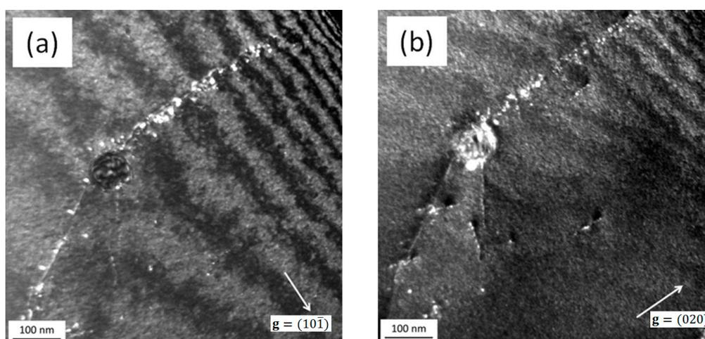
**Figure 3.** TEM weak-beam dark-field images of a dislocation decorated with loops for the Fe-12Cr alloy that was irradiated to 0.6 dpa. (a) Diffraction vector  $\mathbf{g} = (10\bar{1})$ ; (b) same detail,  $\mathbf{g} = (020)$ .
