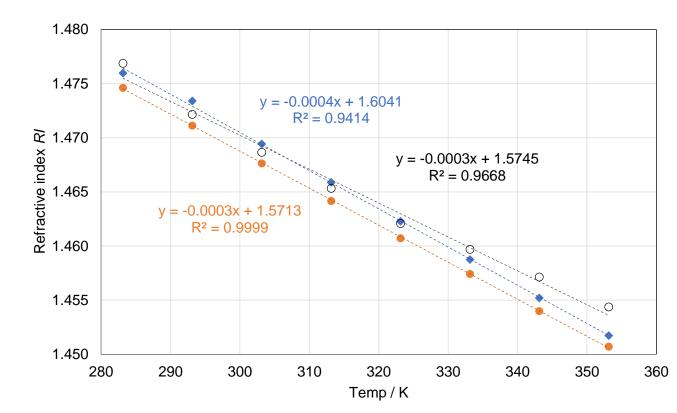
**Figure 2.** Measured refractive index versus temperature for cottonseed oil, epoxidized cottonseed oil and carbonated cottonseed oil. •, CSO; •, ECSO; o, CCSO.
