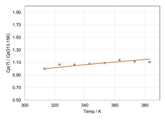
**Figure 11.** Fit of the model to the specific heat capacity experimental data of solution S2. •, Experiment data; —, Model data.
