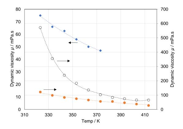
**Figure 4.** Measured dynamic viscosity versus temperature for cottonseed oil, epoxidized cottonseed oil and carbonated cottonseed oil. •, CSO; •, ECSO; o, CCSO.
