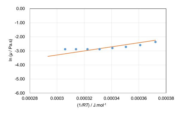
**Figure 10.** Fit of the model to the viscosity experimental data of solution S1. •, Experiment data; —, Model data.
