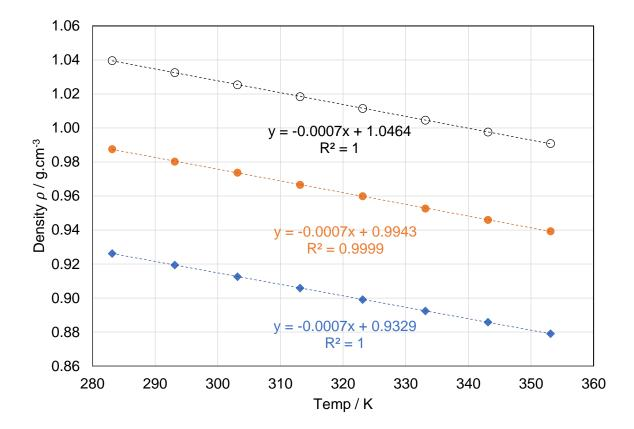
**Figure 3.** Measured density versus temperature for cottonseed oil, epoxidized cottonseed oil and carbonated cottonseed oil. •, CSO; •, ECSO; o, CCSO.
