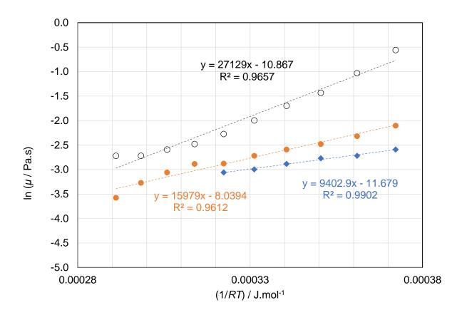
**Figure 5.** Linear correlation between the logarithm of viscosity and 1/RT. ◆, CSO; ●, ECSO; ○,
