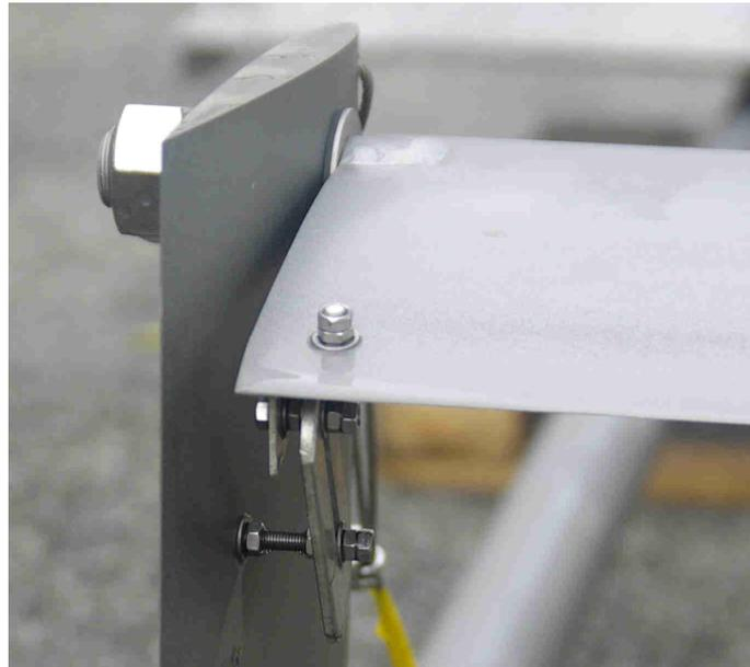
Fig. 6 Adjustment of the stabilizing fin tilt.
