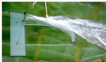
**System for high-frequency simultaneous water sampling at several depths during sailing**
