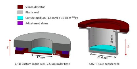
Figure 1. Cross section of the experimental setups. In the first configuration (CH1), a custom made well with a mylar base of  $2.5 \,\mu m$  thickness, was placed 1 mm above a silicon detector. In the second configuration (CH2), the detector was placed above a standard culture well (from 6-well plate) of  $21.6 \, mm$  diameter and  $20 \, mm$  height. The distance between the culture medium surface and the active area of the silicon detector was  $19 \, mm$ .
