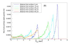
Figure 3. Energy spectra simulated in both configurations (CH1 and CH2) for alpha particles emitted from different depths.
