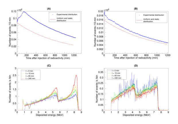
Figure 2. (A) and (B): count rates measured as a function of post-injection time in both configurations and compared to the count rates expected for a static and uniform distribution. (A) corresponds to the CH1 setup and (B) to the CH2 setup. (C) and (D): energy spectra measured at 0, 15, 65 and 245 min respectively in CH1 and CH2 setups (plain lines) and convoluted spectra (bold dashed lines).
