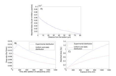
Figure 7. Dose deposited by alpha particles in a  $20 \, \mu m$  thick cylindrical volume of water representing cell culture. A) Dose deposited per emitted  $\alpha$ -particle according to the emission position. B) Dose deposited in  $10 \, minutes$  by the experimental spatial distribution and a uniform and static distribution as a function of time. C) Absorbed dose as a function of exposure time for the experimental and a uniform and static distribution.
