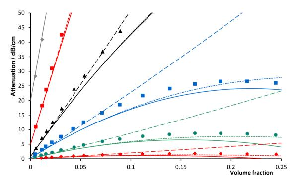
Figure 1. Attenuation as a function of concentration (volume fraction). Symbols: Hipp et al. [3] experiments. Solid lines: from Eq.(3), limited to second order in concentration. Dotted lines: from Eq.(3), up to third order in concentration. Dashed lines: Lloyd and Berry model [2]. The attenuation increases with frequency. Red: 2 MHz. Green: 5 MHz. Blue: 10 MHz. Black: 20 MHz. Red: 50 MHz. Gray: 100 MHz.
