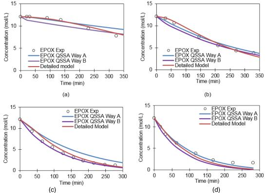
Figure 7– Fit of the detailed and simplified kinetic model with the experimental data at (a)  $60^{\circ}$ C (b)  $70^{\circ}$ C (c)  $80^{\circ}$ C (d)  $90^{\circ}$ C –3 bar of CO<sub>2</sub> and 5% mol of catalyst.
