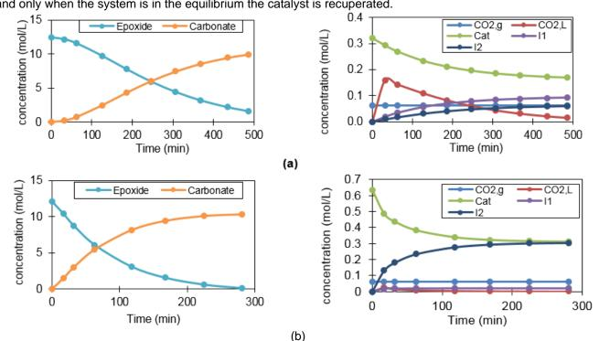
Figure 6 – Concentration profiles of species involving in the reaction of carbon dioxide with epoxides for detailed reaction mechanism – 3 bar of CO<sub>2</sub>, 5% mol of non-metallic catalyst (a) 70°C (b) 90°C
