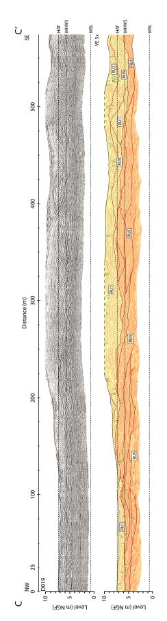
Fig. 12. Ground penetrating radar (GPR) profile C-C' shows south-eastward dipping clinoforms of the barrier unit, overlain by aeolian deposits. Note that the profile is cut off at 10 m Nivellement Général de la France (NGF) to enhance the visualisation of the marine deposits. For the key to the profile, see
