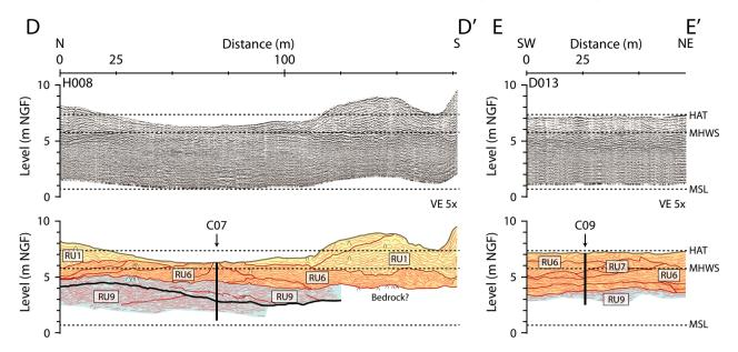
Fig. 13. Ground penetrating radar (GPR) profiles D–D' and E–E'. The bold black line in profile D–D' marks the boundary between older estuarine deposits and younger estuarine and barrier deposits. For the key to the profiles, see Fig. 10. HAT, highest astronomical tide; MHWS, mean high water spring; MSL, mean sea level.
