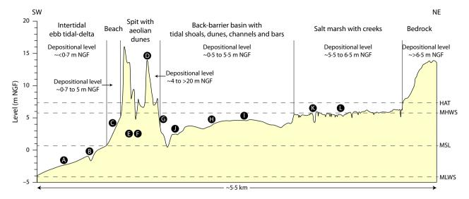
Fig. 4. Schematic cross-shore profile illustrating the main modern depositional environments at the study site and their elevation relative to Nivellement Général de la France (NGF) vertical datum. The levels of highest astronomical tide (HAT), mean high water spring tide (MHWS), mean sea level (MSL) and mean low water spring tide (MLWS) are indicated. The letters (A to L) show the approximate positions of the photographs in Fig. 5.
