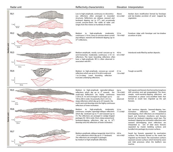
Fig. 9. Radar unit characteristics and geological interpretation. Terminology of reflection characteristics is based on Neal (2004). Directions of dips are apparent measures and inclinations are given without vertical exaggeration. The amplitudes are all relative due to corrections applied during processing.
