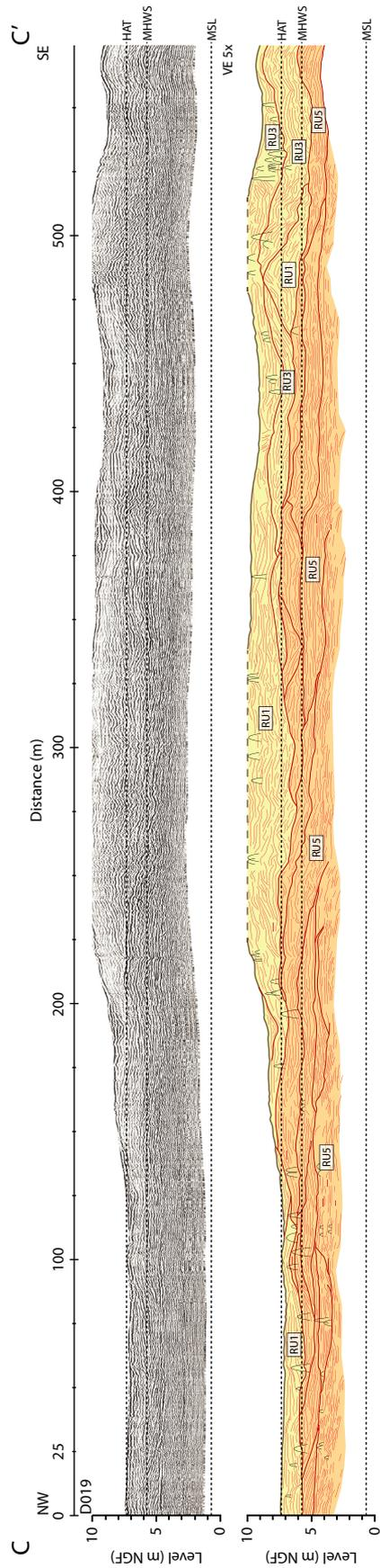
**Fig. 12.** Ground penetrating radar (GPR) profile C–C' shows south-eastward dipping clinofolds of the barrier unit, overlain by aeolian deposits. Note that the profile is cut off at 10 m Nivellement Général de la France (NGF) to enhance the visualisation of the marine deposits. For the key to the profile, see Fig. 10.
