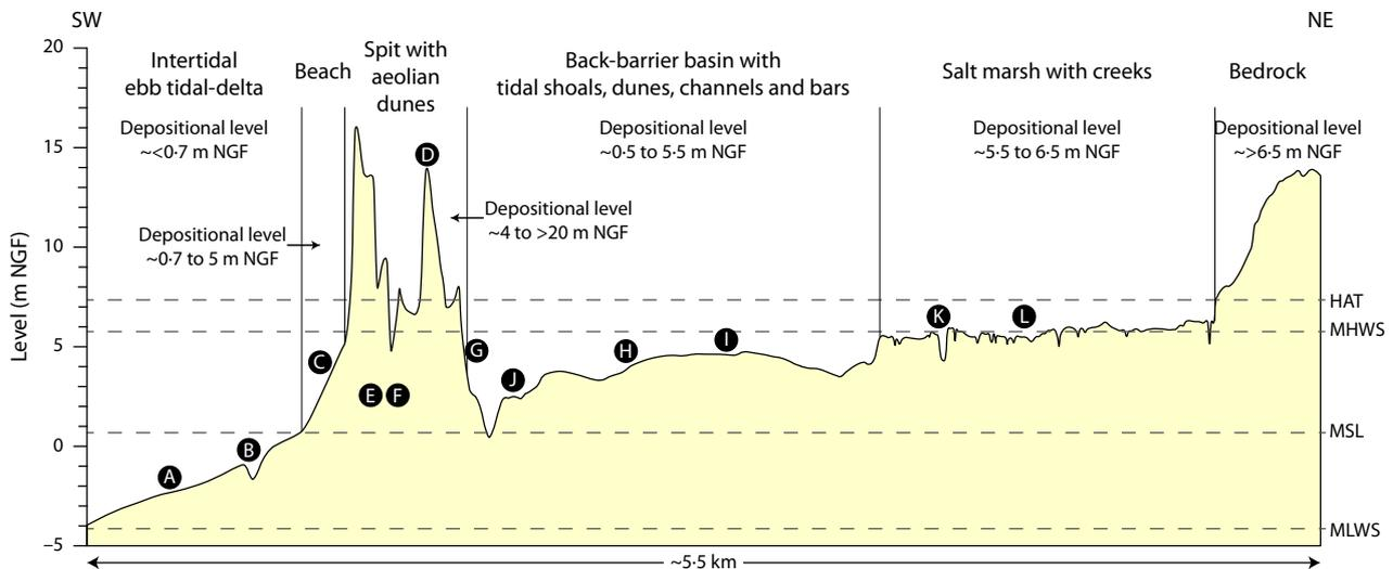
**Fig. 4.** Schematic cross-shore profile illustrating the main modern depositional environments at the study site and their elevation relative to Nivellement Général de la France (NGF) vertical datum. The levels of highest astronomical tide (HAT), mean high water spring tide (MHWS), mean sea level (MSL) and mean low water spring tide (MLWS) are indicated. The letters (A to L) show the approximate positions of the photographs in Fig. 5.
