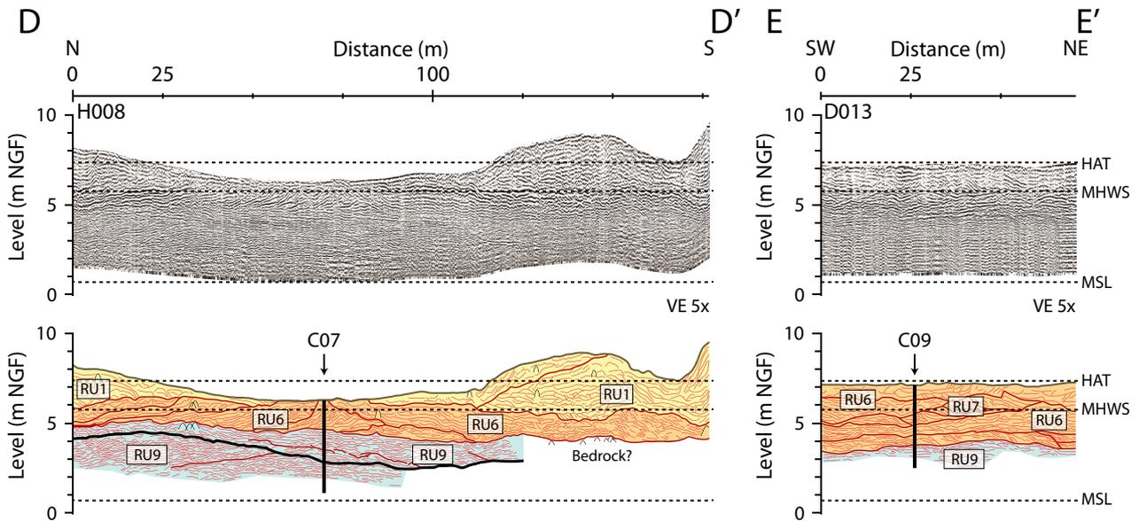
**Fig. 13.** Ground penetrating radar (GPR) profiles D–D' and E–E'. The bold black line in profile D–D' marks the boundary between older estuarine deposits and younger estuarine and barrier deposits. For the key to the profiles, see Fig. 10. HAT, highest astronomical tide; MHWS, mean high water spring; MSL, mean sea level.
