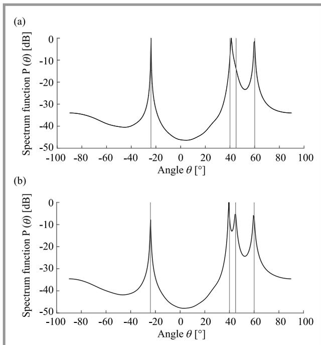
**Fig. 8.** Propagator spectrum: (a) before – 13 elements and (b) after – 14 elements.
