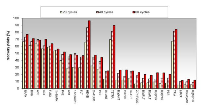
Figure 1. Soxhlet extraction of a mixture of spiked PAHs, nitro-PAHs and n-alkanes from 100 mg of diesel particulate matter, blown-off from a diesel particulate filter after an European NEDC driving cycle test. Extraction conditions: reflux of 120 mL methylene chloride, each cycle representing approximately 8 minutes.
