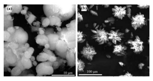
**Figure 2** SEM images of the as-synthesized samples DFZ-64C (a) and DFZ-64D (b).
