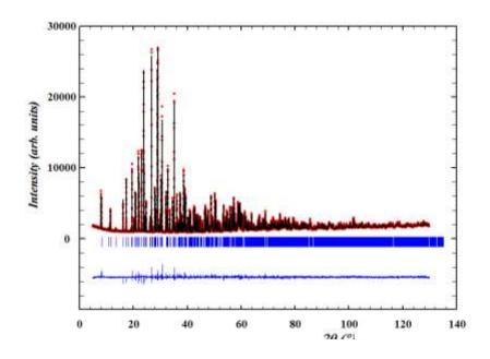
**Figure 3** PXRD diagram of DFZ-64C-LT at 20°C (Cu–Kα1 radiation; 1.5406Å) with observed (dots), calculated (solid line), Bragg reflections (ticks), and difference profiles (bottom line) obtained after Rietveld refinements.
