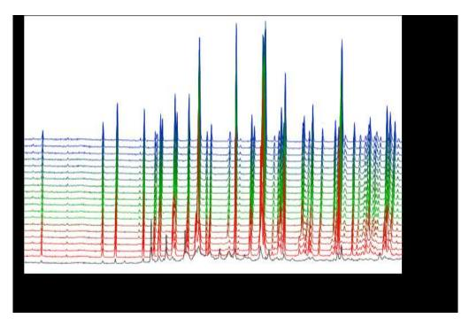
Figure 8 Temperature-programmed in-situ XRD patterns of sample DFZ-64C.
