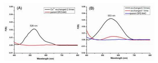
**Figure 11** The UV-VIS spectra of sample DFZ-64C after Co<sup>2+</sup> exchange in 0.05 M Co(Ac)<sub>2</sub> solution (A, 50 °C, 4h) and Cu<sup>2+</sup> exchange in 0.05 M Cu(Ac)<sub>2</sub> solution (B, 50 °C, 4h).
