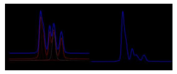
Figure 6 <sup>31</sup>P MAS (left) and <sup>1</sup>H-<sup>31</sup>P CP MAS NMR spectra (right) of sample DFZ-64C.
