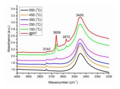
**Figure 10** Analysis of the -OH stretching mode of sample DFZ-64C by temperature-programmed in-situ FTIR spectroscopy.
