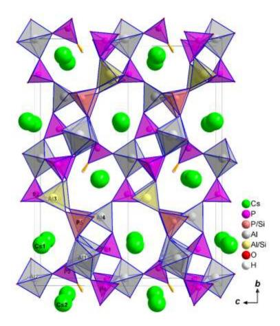
**Figure 4** Structure projection of the (bc) plane; 8-MR channels occupied by  $Cs^+$  cations are observed along the a axis.
