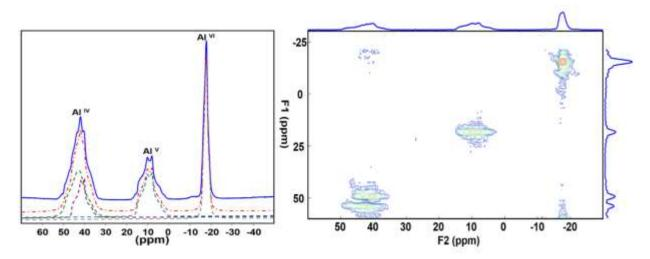
**Figure 5** 1d <sup>27</sup>Al MAS NMR spectra (left) and 2d <sup>27</sup>Al MQ MAS NMR spectra (right) of sample DFZ-64C
