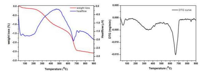
**Figure 7** TG-DSC analysis curves of sample DFZ-64C: TGA and heat flow curves (left) and DTG curve (right).
