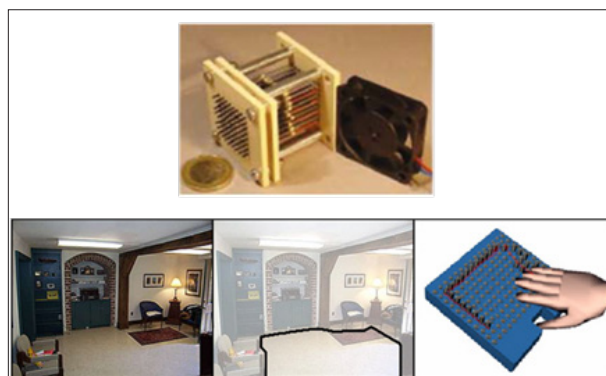
Figure 2: Illustration of the developed scene representation (bottom row) and device (top row). Images of the scene, acquired with a stereo rig, are processed to create a 2D tactile map (right image). This simplified representation (tactile gist) shows dynamically the accessible and non-accessible parts of the environment delimited by raised taxels. The origin of the Euclidian reference frame is attached to the tactile map and is materialized by a notch in one of the device borders. The stimulation device is a Braille matrix of 8 by 8 shape memory alloys based taxels [4,5,6].
