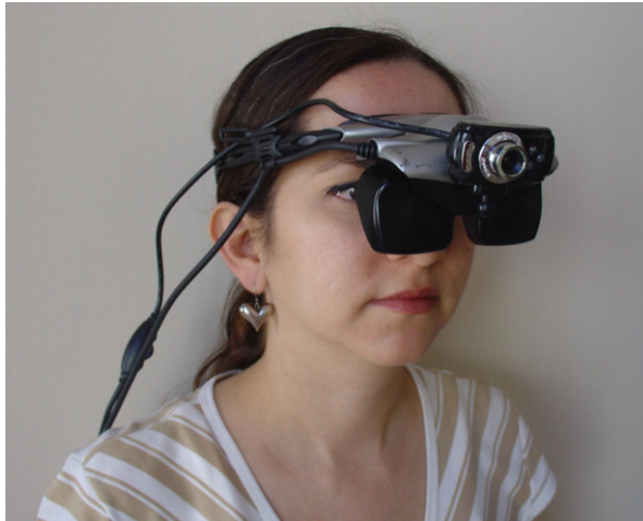
Fig. 1. Visual impairment simulator: (a) Design and (b) prototype.
