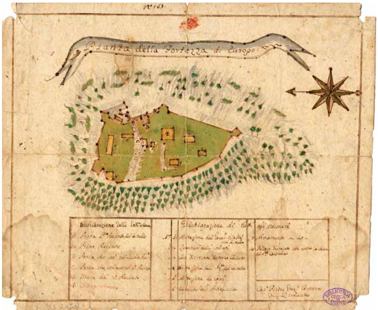
11. Pietro Gregorio Carrara, 'Pianta della fortezza di Osoppo', mid-18th century. Although drawn some time after the construction of the fortress was completed, this plan shows how the rocca di Osoppo's natural defences were reinforced with walls and bastions. Within the fortress can be seen the church at the centre (shown by a cross), several residential buildings to the south, and military buildings to the north. To the northeast can be identified the terrace on which Giulio Savorgnan's funerary monument, not shown on this plan, was built.
