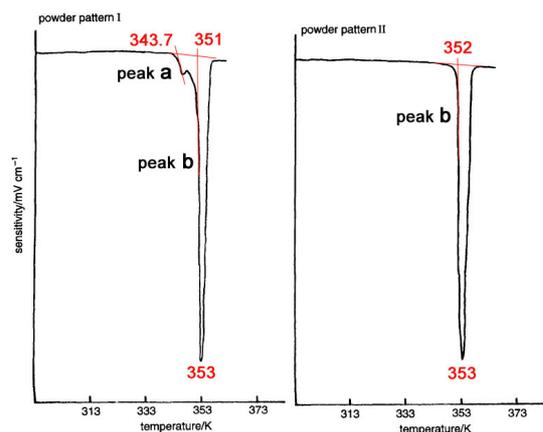
**Figure S2.** DSC curves by Gallagher et al. for the orthorhombic (left-hand panel) and monoclinic (right-hand panel) polymorphs of 2,4,6-trinitrotoluene [9].
