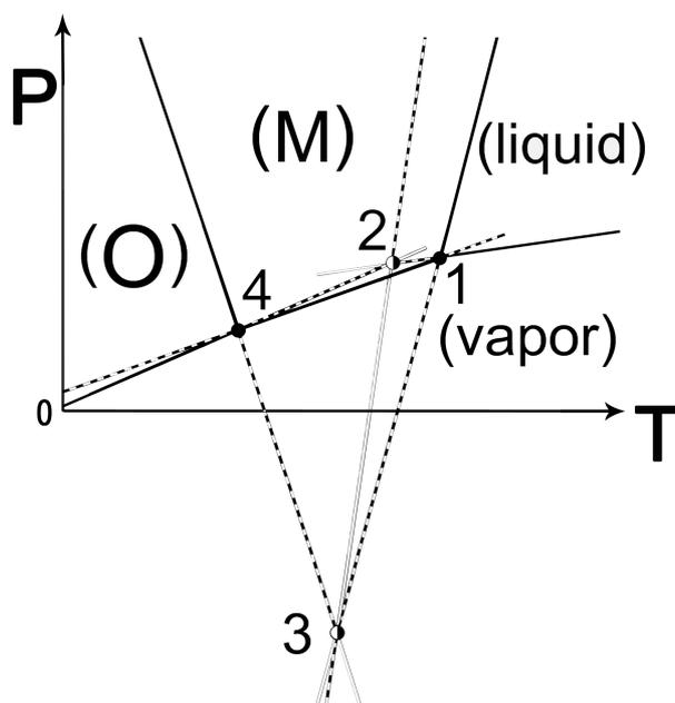
**Figure 2.** Topological pressure-temperature phase diagram of TNT representing the stability regions of forms O and M, the liquid (L) and the vapor (V) phase. Triple points: 1: M-L-V, 2: O-L-V, 3: O-M-L, 4: O-M-V. Stability ranking: solid black lines: stable, dashed lines: metastable, white lines: supermetastable
