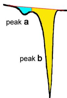
**Figure S4.** Delimitation of peaks 'a' and 'b' for Figure 1 in the text and Figures S2 and S3 in the supplementary materials. The yellow area is ascribed to the heat of fusion of the monoclinic polymorph and the blue area to the transition of form O into form M.
