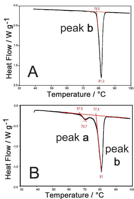
**Figure S3.** DSC curves of TNT published by Vrcelj et al. [1, 2]: panel A monoclinic form (M) and panel B orthorhombic form (O). Peak 'a' = O→M (onset at 340.6 K), peak 'b' = M→liquid (onset at 351-352 K).
