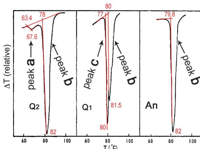
**Figure 1.** Differential thermal analysis curves of TNT modifications recorded at  $10 \text{ K min}^{-1}$  by Grabar et al. [18]. Specimens Q1 and Q2 correspond to the orthorhombic (O) modification (see Table T2) and specimen An is identified by the authors as being the monoclinic (M) polymorph. Peak **a** = O→M (onset at 336.6 K), peaks **c** + **b** = O→liquid→M→liquid, peak **b** = M→liquid (onset at 353 K). Figures from reference [18] and adapted for this paper.
