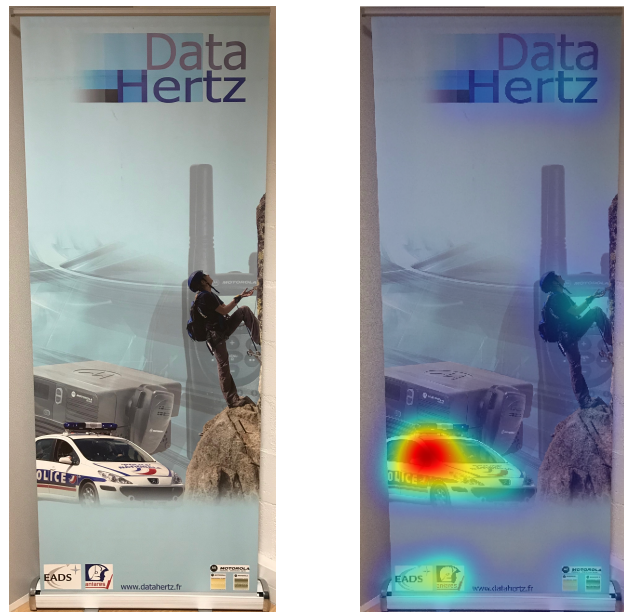
Fig. 2. Example of a saliency map: left – original image, right – saliency map (overlay), obtained using Itti et al. algorithm [26]. The saliency values increase here from blue to red.
