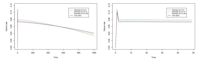
Fig. 3 Failure rate estimation: all the trajectory (up) and a zoom (down)  $% \left( {{{\mathbf{F}}_{\mathrm{s}}}^{\mathrm{T}}} \right)$
