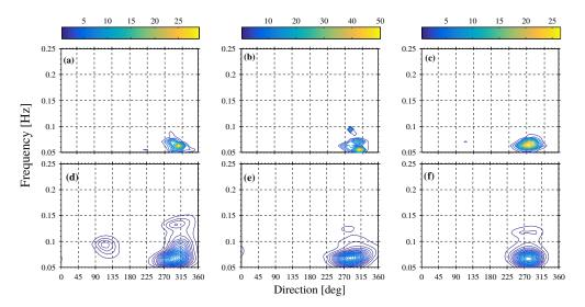
**Figure 5.** Radar and in situ estimates of wave directional spectra on 21 October 2012 at 1000 UTC. The upper panels show the results obtained from the in situ measurements, and the bottom panels show the radar estimates: ADCP-E spectra (a,d); and ADCP-W (b,e). Wave buoy (c,f). The colorbar represents the directional energy density  $(m^2/Hz/deg)$ .
