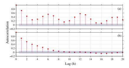
**Figure 11.** Autocorrelation function of the time series of the differences between directional spread measured at two locations: (a) autocorrelation of differences between the wave buoy and the ADCP-E directional spread; and (b) autocorrelation of the differences between the radar directional spread estimates obtained at the buoy and ADCP-E sites. The confidence bounds are shown in blue.
