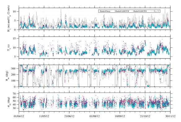
**Figure 2.** Radar wave parameters co-located with the wave buoy (red star), the ADCP-W (dark blue dots) and ADCP-E (light blue crosses) from April to November 2012 (a) significant wave height and wind speed (grey line); (b) energy period; (c) wave direction (direction of approach) and wind direction (grey line); and (d) mean directional spreading.
