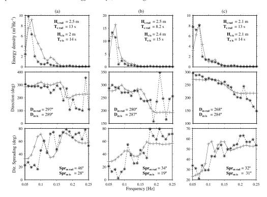
**Figure 6.** Radar and in situ estimates of one-dimensional spectra, mean direction and directional spreading as a function of frequency on 21 October 2012 at 1000 UTC: (a) ADCP-E (dashed black line and \*) and radar (grey line and +); (b) ADCP-W (dashed black line and \*) and radar (grey line and +); and (c) buoy (dashed black line and \*) and radar (grey line and +).
