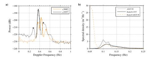
**Figure 12.** Radar measurement affected by antenna sidelobes: (a) The Doppler spectra measured at  $14^{\circ}$  (black line) and  $45^{\circ}$  (orange line) from Perranporth's normal. The first-order region of each spectrum is emphasized with a full line. The stars indicate the identified second order peaks. (b) The frequency spectra obtained at the same two cells, and measured by the ADCP-W, located at cell 3682.
