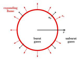
Figure 13: Schematic of a spherical expanding flame.
