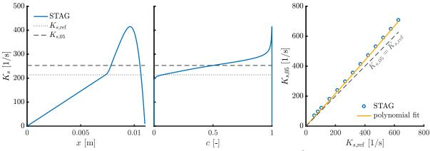
Figure 5: Strain rate  $K_s$  for a lean H<sub>2</sub>-air stagnation flame with  $K_{s,ref} = 214 \,\mathrm{s}^{-1}$  versus the physical space coordinate (left) and the normalized progress variable c (middle). For the premixed flamelet model  $K_{s,05}$  is prescribed which is expressed as a function of  $K_{s,ref}$  to facilitate a comparison of the premixed flamelet model to experiments (right).
