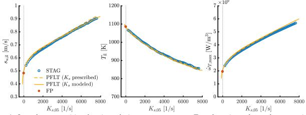
Figure 9: Inner layer quantities: burning velocity  $s_{u,\mathrm{il}}$ , temperature  $T_{\mathrm{il}}$  and maximum heat release rate  $\dot{\omega}_{T,\mathrm{max}}$  as functions of strain for lean H<sub>2</sub>-air flames ( $\varphi=0.5,\ T_u=298\,\mathrm{K}$ ). The progress variable is defined as  $Y_c=Y_{\mathrm{H_2O}}-Y_{\mathrm{H_2}}-Y_{\mathrm{O_2}}$  in the flamelet calculations.
