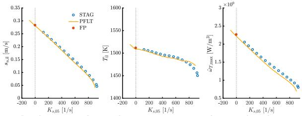
Figure 10: Inner layer quantities burning velocity  $s_{u,\mathrm{il}}$ , temperature  $T_{\mathrm{il}}$  and maximum heat release rate  $\dot{\omega}_{T,\mathrm{max}}$  as functions of strain for lean  $\mathrm{C_2H_5OH}$ -air flames ( $\varphi=0.7,\,T_u=363\,\mathrm{K}$ ). The progress variable is defined as  $Y_c=Y_{\mathrm{CO_2}}+Y_{\mathrm{H_2O}}+10\,Y_{\mathrm{H_2}}-Y_{\mathrm{O_2}}$  in the flamelet calculations.
