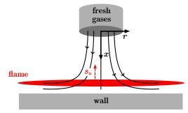
Figure 3: Schematic of a planar stagnation flame.
