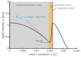
Figure 4: Flow field of the stagnation flame with the reference flame speed  $s_{u,ref}$  and the reference strain rate  $K_{s,ref}$ , evaluated from the steepest velocity gradient upstream of the flame. Recreated according to Ref. [36].
