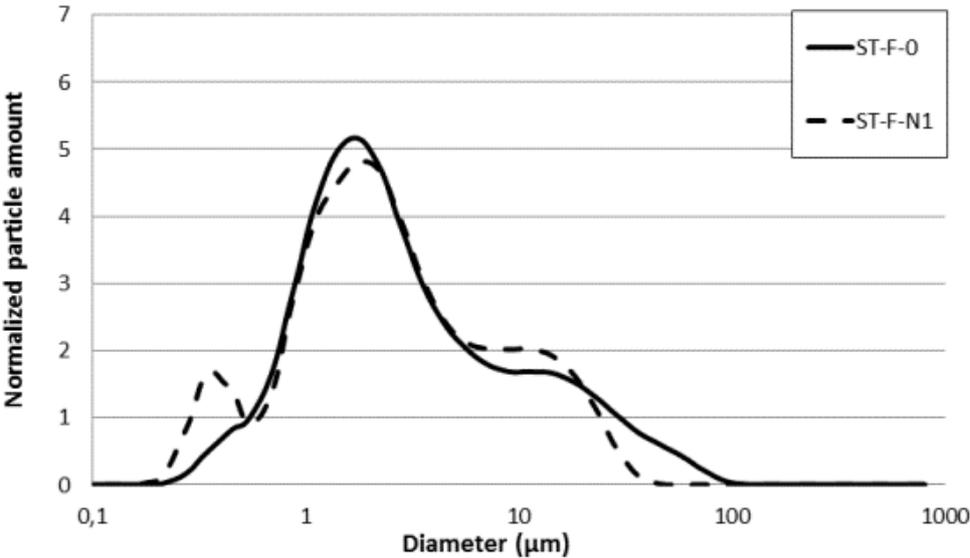
Figure 5: Particle size distributions given in volume particle of sterilized emulsions.
