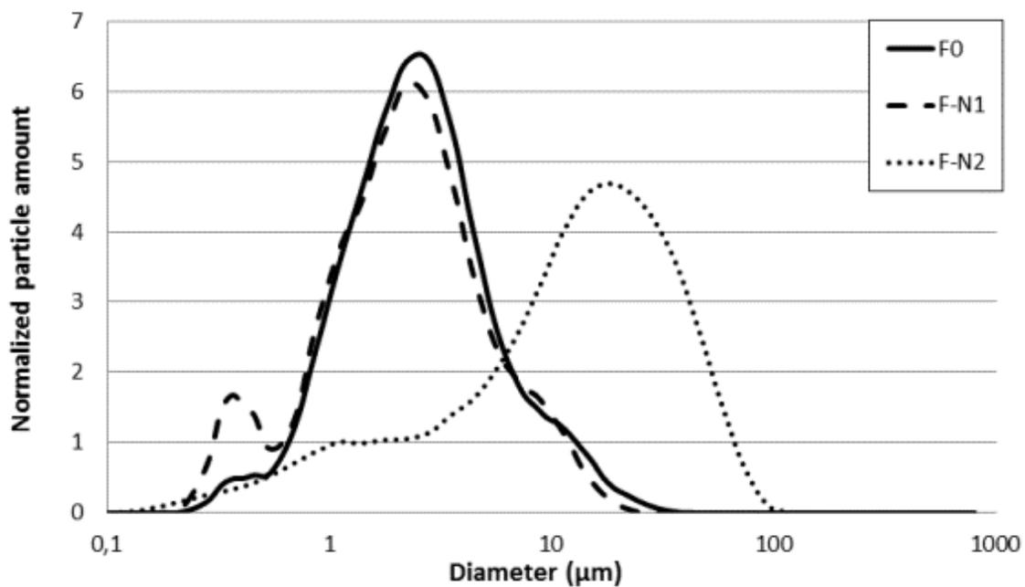
Figure 1: Particle size distributions given in volume particle of fresh emulsions.
