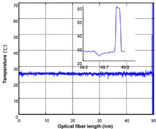
Figure 6. Temperature curve of the 50 km sensing fiber.
