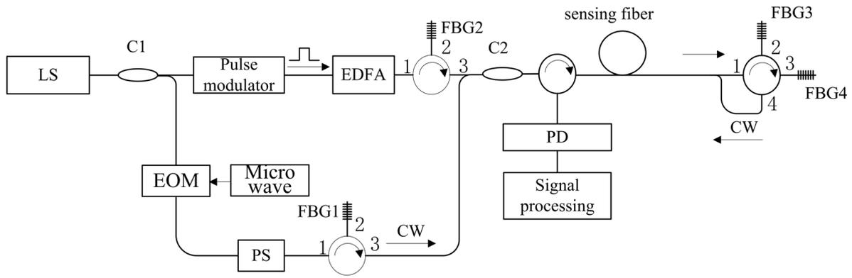
Figure 1. Experimental setup of a 50 km cascading FBG-based single-ended BOTDA.
