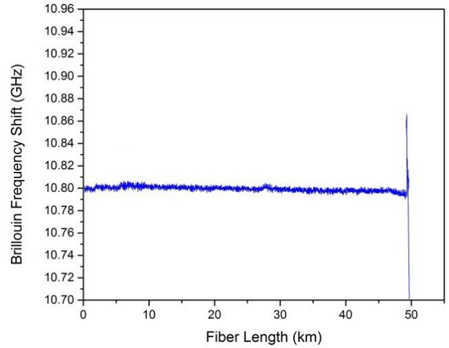
Figure 3. The measured BFS versus the fiber length.
