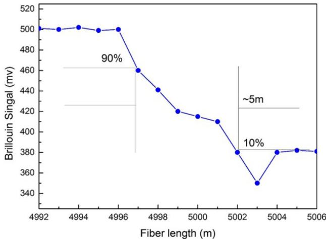
Figure 5. BFS versus distance near the end of the fiber.
