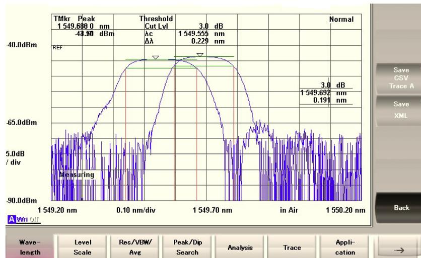
Figure 2. The measured spectra of FBG3 and FBG4.
