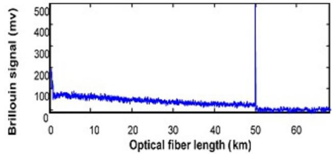
Figure 4. The Brillouin signal when the modulation frequency is at 10.796 GHz.
