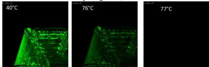
Fig. 2 SHG-M pictures upon heating of ultrapure phenanthrene single-crystal.
