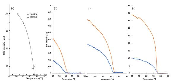
Fig. 3 TR-SHG curves of phenanthrene adapted from [7] (a) and for 90% (b), 98% (c) and ultrapure (d) grades.
