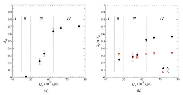
**Figure 5**. Internal flow: cavitation plume area  $A_B$  (a) and centroid coordinates ( $X_B$ ,  $Y_B$ ) (b) as a function of the flow rate. Error bars represent the standard deviation of the quantities over the image series.
