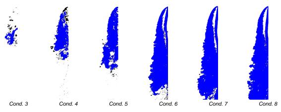
Figure 4. Internal flow: segmented image example for conditions 3 to 8. The cavitation plume is shown in blue.
