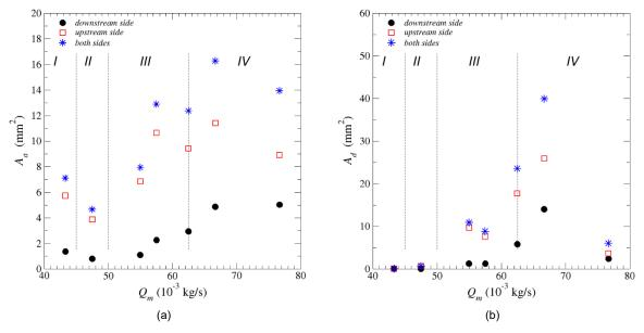
Figure 9. External flow: a - primary atomization zone and b - droplet probability areas as functions of flow rate.
