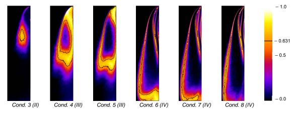
**Figure 6**. Internal flow: entropy maps for conditions 3 to 8 (regimes indicated in brackets). Correspondence between colours and entropy values are given in the right column. The black lines delimits the 3-state regions (E<sub>3</sub>=0.631).
