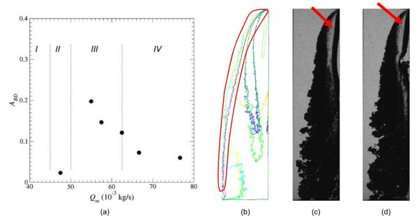
**Figure 7**. Internal flow: a - Normalized area of the bubble detachment region A<sub>BD</sub> as a function of the flow rate; b – non-null entropy contours superimposed for the condition 3 to 8; c,d – images of the flow in condition 8.
