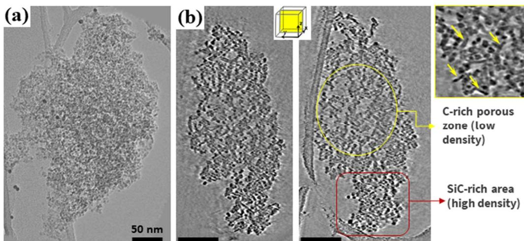
**Figure 10.** Electron tomography of the HF-etched SiBOC sample. (a) TEM micrograph acquired during the series acquisition. (b) General and detailed slices redrawn from the reconstructed volume identifying the high porosity of the C-rich areas and the 3D agglomeration of the SiC nanoparticles.
