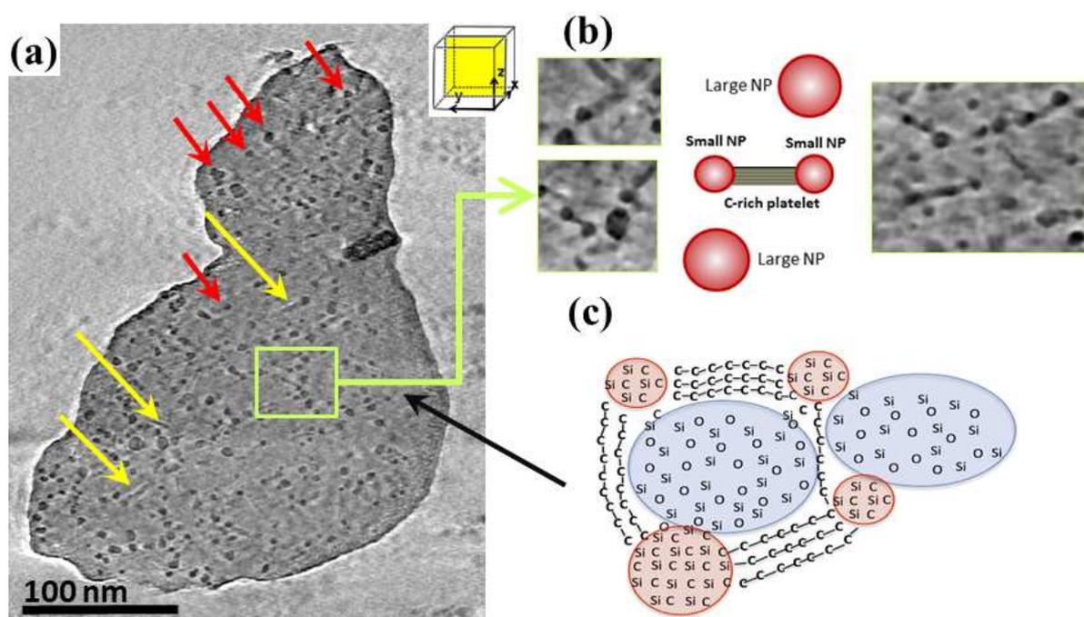
**Figure 6.** (a) Typical slice redrawn from the reconstructed volume; the yellow arrows point to a carbon rich and the red arrows point to SiC NPs areas embedded in SiO<sub>2</sub>-based glass (light grey). (b) Higher magnification slices of the C-rich platelets bridging the small SiC NPs located in the close vicinity of larger NPs. (c) Schematic representation of the ordering and bonding within the chemically different domains.
