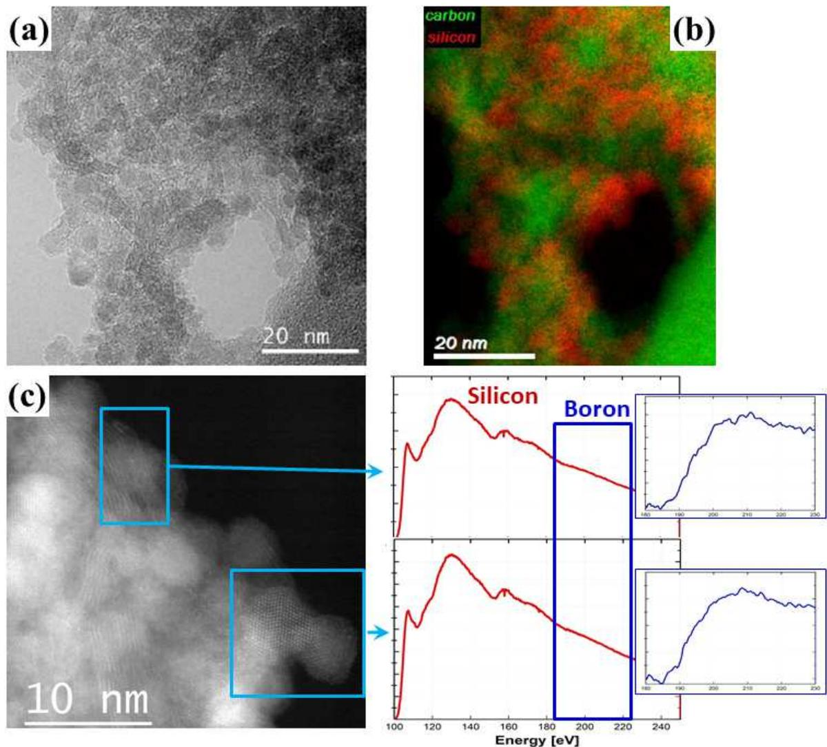
**Figure 9.** (a) Typical zero loss energy filtered TEM (elastically scattered electrons) micrograph and (b) superposition of the C and Si maps of a representative area within the HF treated SiBOC glass. (c) STEM-HAADF image and the selection of the regions chosen for the acquisition of cumulative energy loss spectra displayed on the right side; the insets represent the B spectra (rectangle in the Si signal) after background removal.
