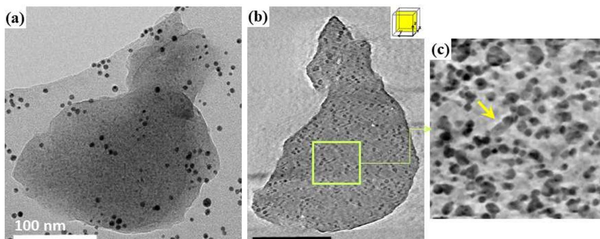
**Figure 5.** Electron tomography of the parent SiBOC sample. (a) As-acquired TEM micrograph extracted from the raw series of images (the dark particles are Au fiducials used for the images fine alignment). (b) General and (c) detailed slices redrawn from the reconstructed volume; the yellow arrow points to a carbon rich area embedded in the SiO<sub>2</sub>-based matrix (light grey) and SiC NPs (darker particles). Scale bar in (b): 100 nm
