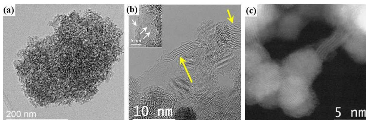
**Figure 7.** TEM micrographs of the SiBOC glasses after HF etching treatment. (a) General aspect of one agglomerate constituted by (b) SiC nanograins with sizes smaller than 10 nm and graphitic structures indicated by the yellow arrows. The white arrows in the HR image from the inset point to surface defects commonly identified on the surface of graphene sheets (c) HR STEM HAADF image of nanoparticles connected by graphitic structures.
