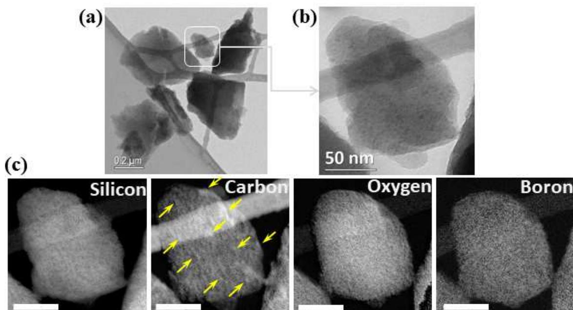
**Figure 4.** (a) General and (b) detailed views of the SiBOC grains prior to the HF treatment. (c) Chemical maps of the elements of interest: Silicon Carbon, Oxygen and Boron, acquired in EFTEM; scalebar: 50 nm.
