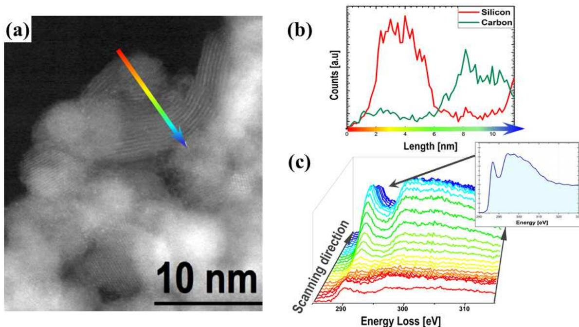
**Figure 8.** Spectrum imaging analysis (STEM-EELS) of the SiBOC glass after HF treatment. (a) STEM-HAADF micrograph of the region chosen for the line scan along the direction indicated. (b) The variation of the C and Si content and (c) the Carbon (K edge) fine structure evolution along the scanning direction. Note: the colors in the graphical representation above were randomly chosen.
