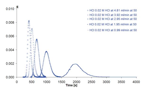
Fig.2. E-curves at 30°C by using HCl as a tracer.
