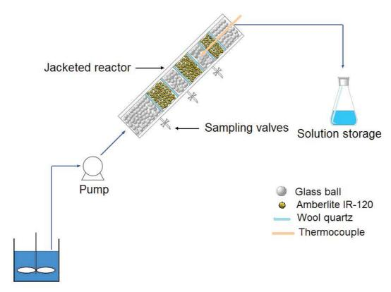
Pre-mixing carboxylic acid and hydrogen peroxide solution
