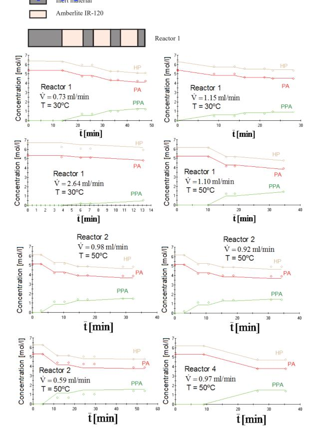
Fig. 12. Fit of the plug flow model to the perhydrolysis experiments of propionic acid.
