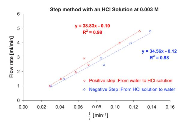
Fig. 9. Flow rate versus  $\frac{1}{\bar{t}}$  in the reactor 4 at 50°C.
