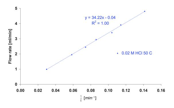
Fig. 3. Flow rate versus the inverse of the mean residence time at 50°C for reactor 4.
