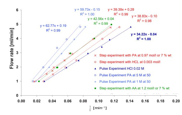
Fig. 10. Flow rate versus the reciprocal value of the mean residence time for reactor 4 at 50°C.
