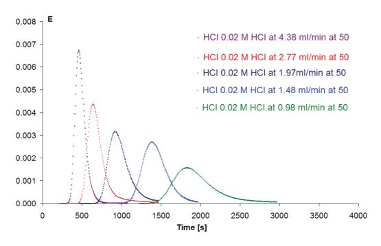
Fig. 6. E-curves for reactor 3 at different flow rates.
