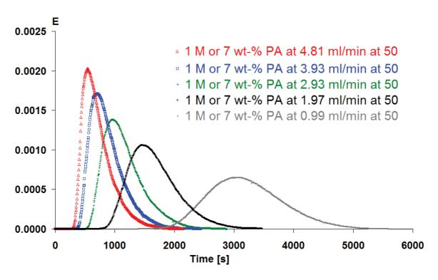
Fig. 7. E-curves for reactor 4 at 50°C using a 1 M of propionic acid solution.
