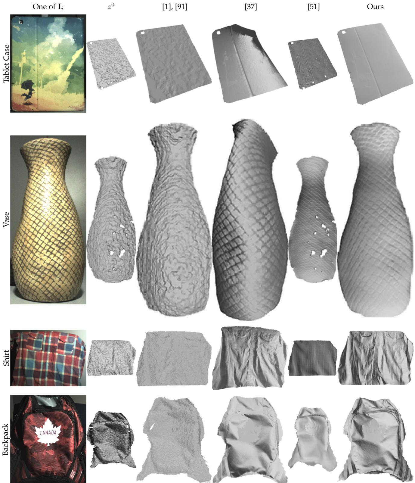
Fig. 26: Comparison between the proposed multi-shot method and the state-of-the-art, on real-world datasets captured using an Asus Xtion Pro Live camera. These results confirm the conclusion of the synthetic experiments in Figure 25.
