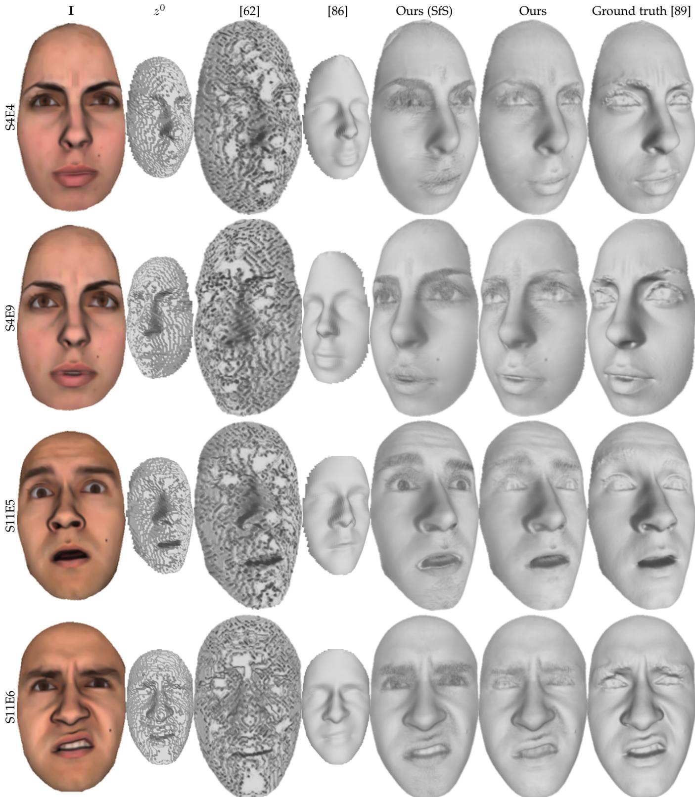
Fig. 19: Qualitative comparison of the results obtained using the deep learning-based depth super-resolution technique from [62], the deep learning-based shape-from-shading approach from [86], the proposed variational approach to shape-from-shading (denoted by SfS), and the proposed combination of deep learning and variational methods. The latter seems the most effective, and this is confirmed by the quantitative evaluation provided in Table 3.
