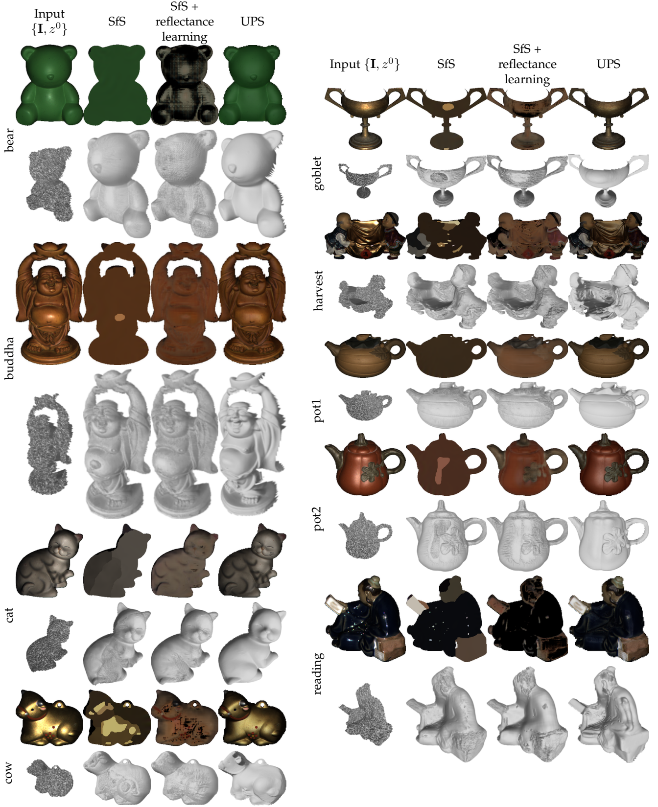
Fig. 28: Comparison of the albedo and high-resolution depth maps estimated by the proposed variational approach to shape-from-shading (SfS), the combination of SfS and deep reflectance learning, and the uncalibrated photometric stereo (UPS)-based approach, on the DiLiGenT dataset [41]. For quantitative evaluation, we refer the reader to Tables 2, 4 and 6.
