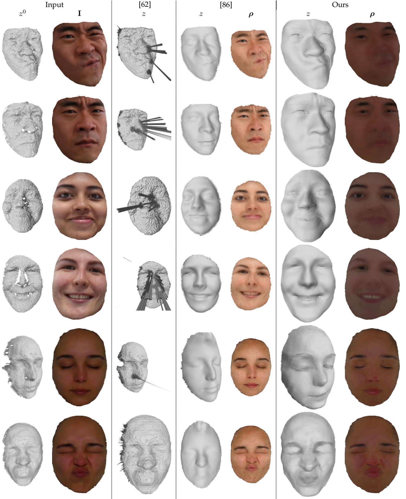
Fig. 20: Qualitative comparison of our reflectance learning-based results against state-of-the-art methods, on six RGB-D frames of human faces which we captured using an Intel RealSense D415 camera (scaling factor of 4). Our method provides the most detailed 3D-reconstructions.
