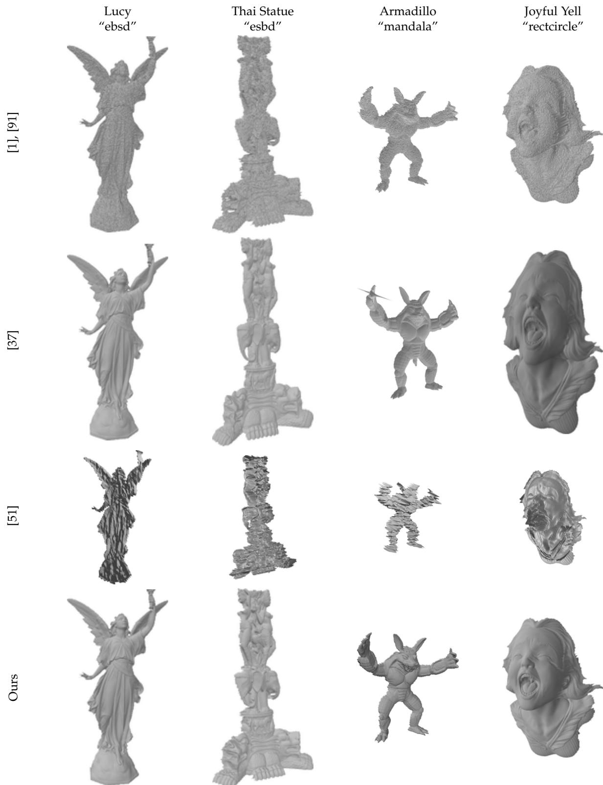
Fig. 25: Qualitative comparison of our multi-shot approach against state-of-the-art methods, on four synthetic datasets (scaling factor of 4). Image-based depth super-resolution adapted from [1], [91] results in noisy geometry, uncalibrated photometric stereo results from [37] are slightly flattened due to the underlying bas-relief ambiguity, and RGB-D fusion [51] of the low-resolution data is not really successful here. In comparison, the results of the proposed method are extremely satisfactory.
